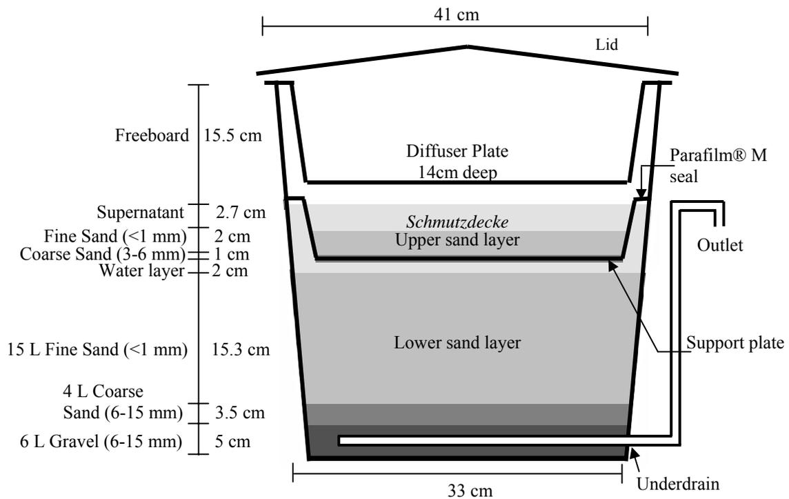
**Figure 6-5 Dual sand layer biosand filter (BSF B)**
