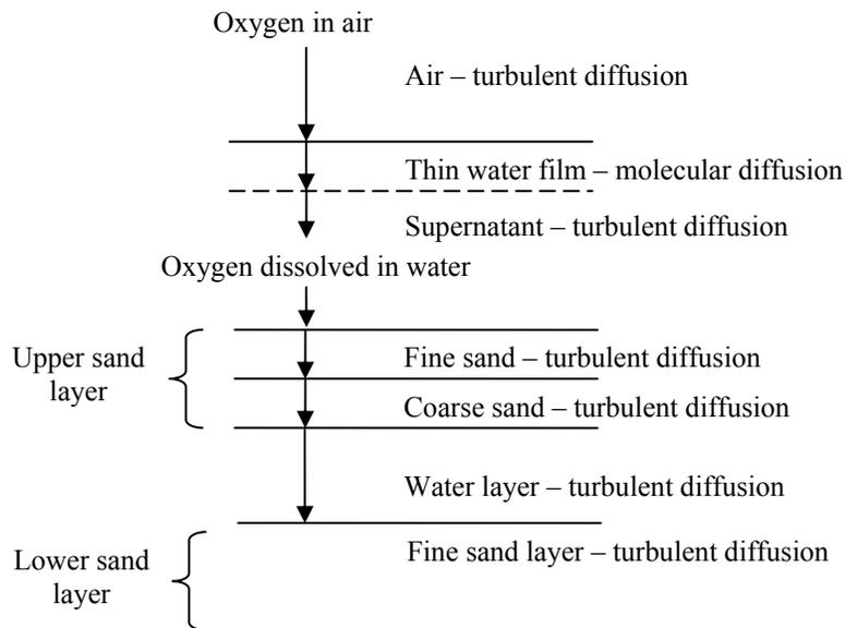
**Figure 6-3 Oxygen diffusion pathway in a dual sand layer BSF**
