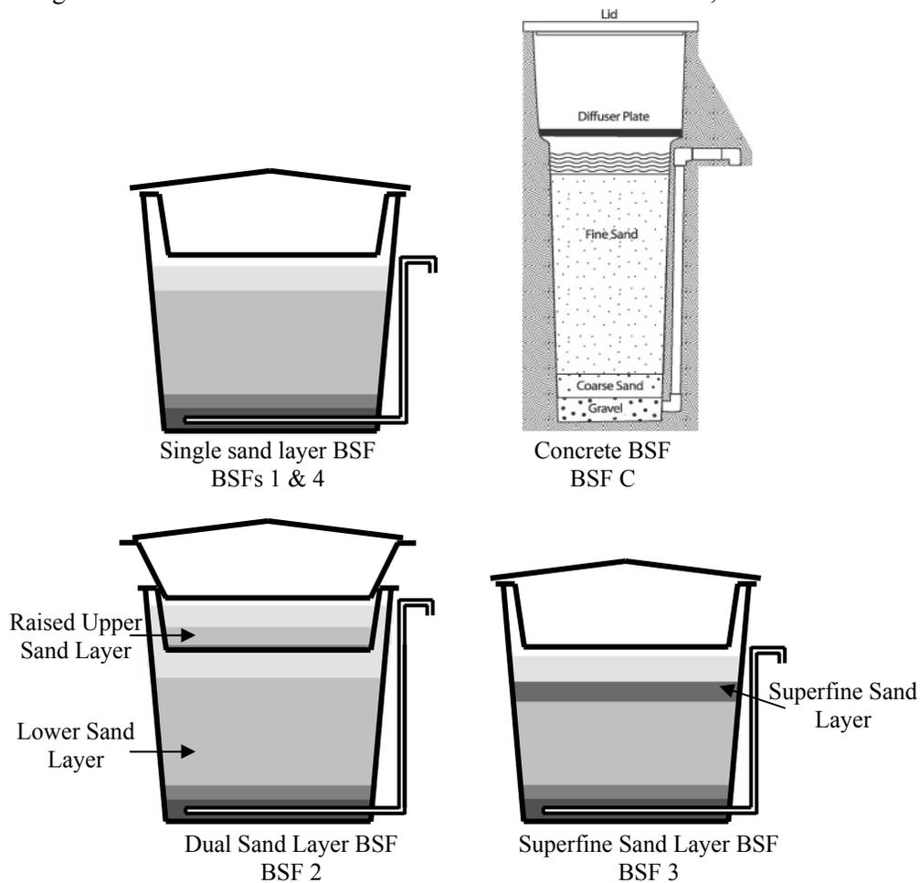
**Figure 5-6 Biosand filter designs tested in Tamale, Ghana**
