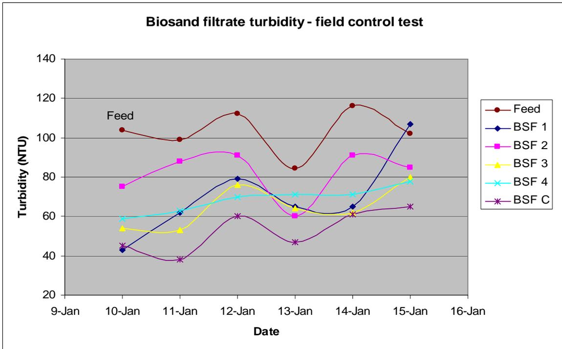
**Figure 5-12 BSF influent and effluent turbidity results, control tests**
