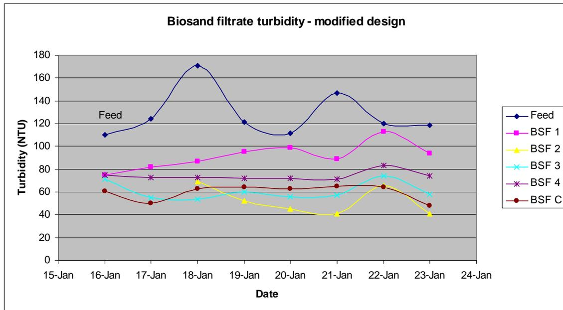
**Figure 5-15 BSF influent and effluent turbidity, modified operation**
