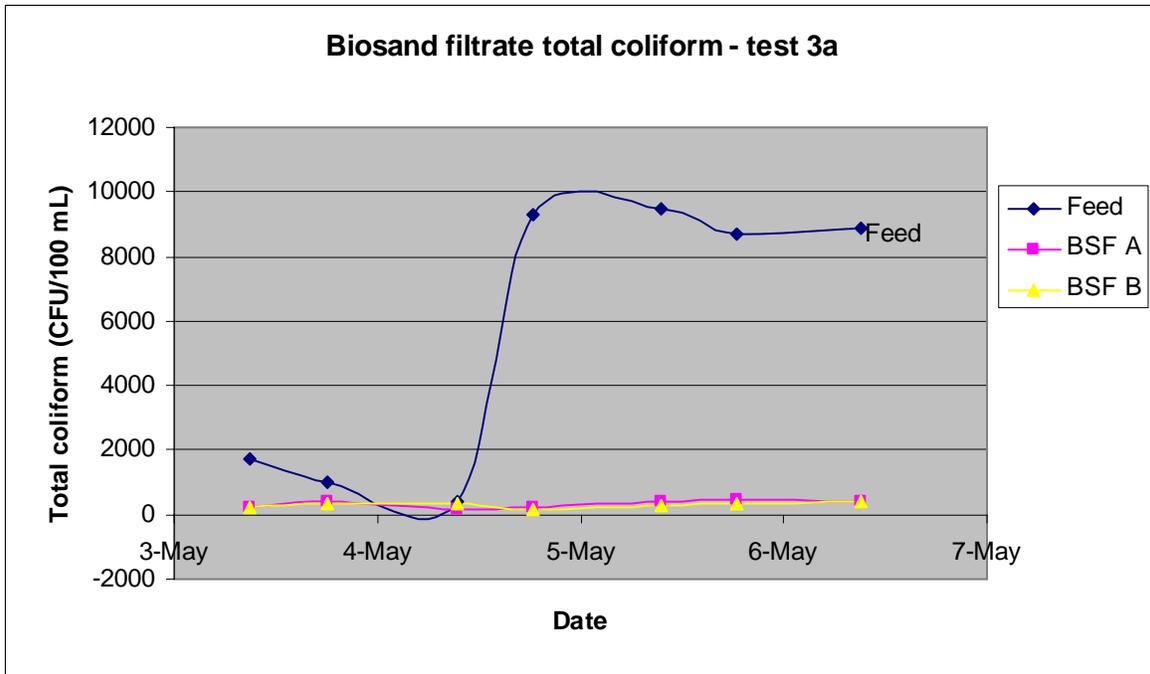
**Figure 6-21 Total coliform counts in BSF influent and effluent, test 3a**
