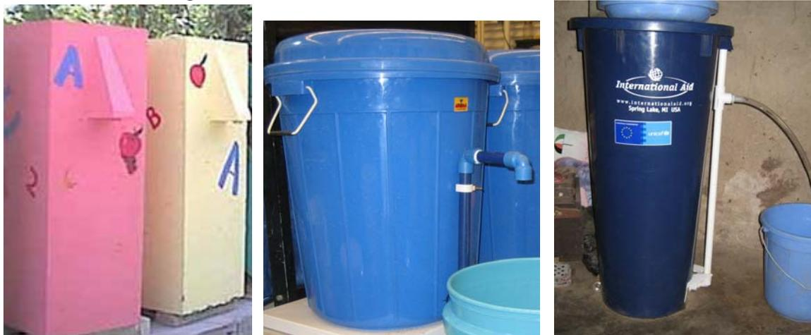
**Figure 3-3 BSFs: a) CAWST design, b) Kanchan™ design, and c) HydrAid filter**
