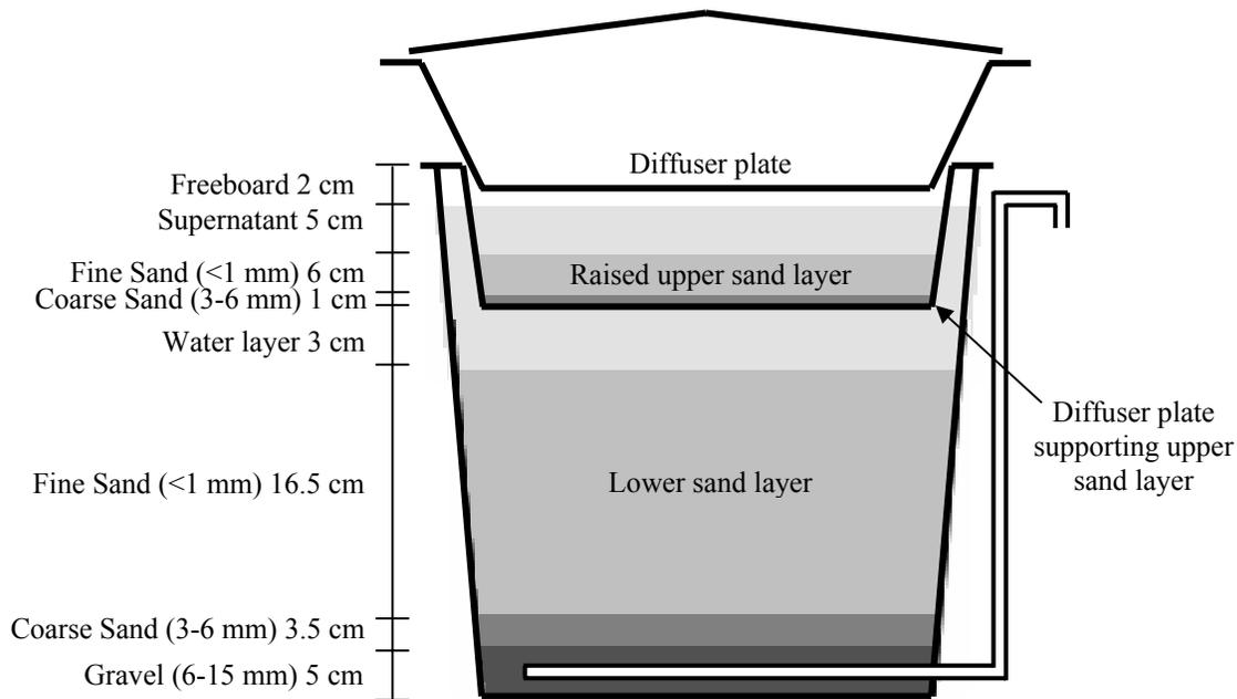
**Figure 5-3 Biosand filter with dual sand layers**
