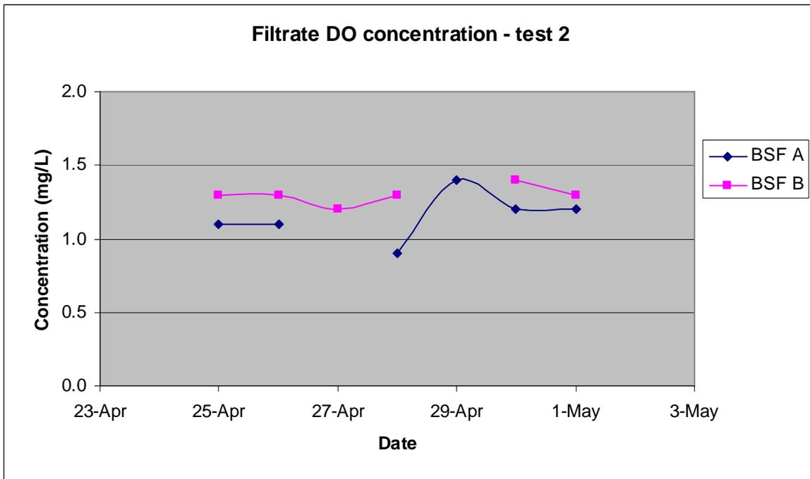
**Figure 6-18 Dissolved oxygen concentrations in the filtrate, test 2**
