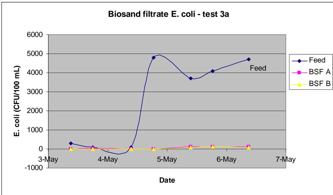
**Figure 6-20** *E. coli* counts in BSF influent and effluent, test 3a
