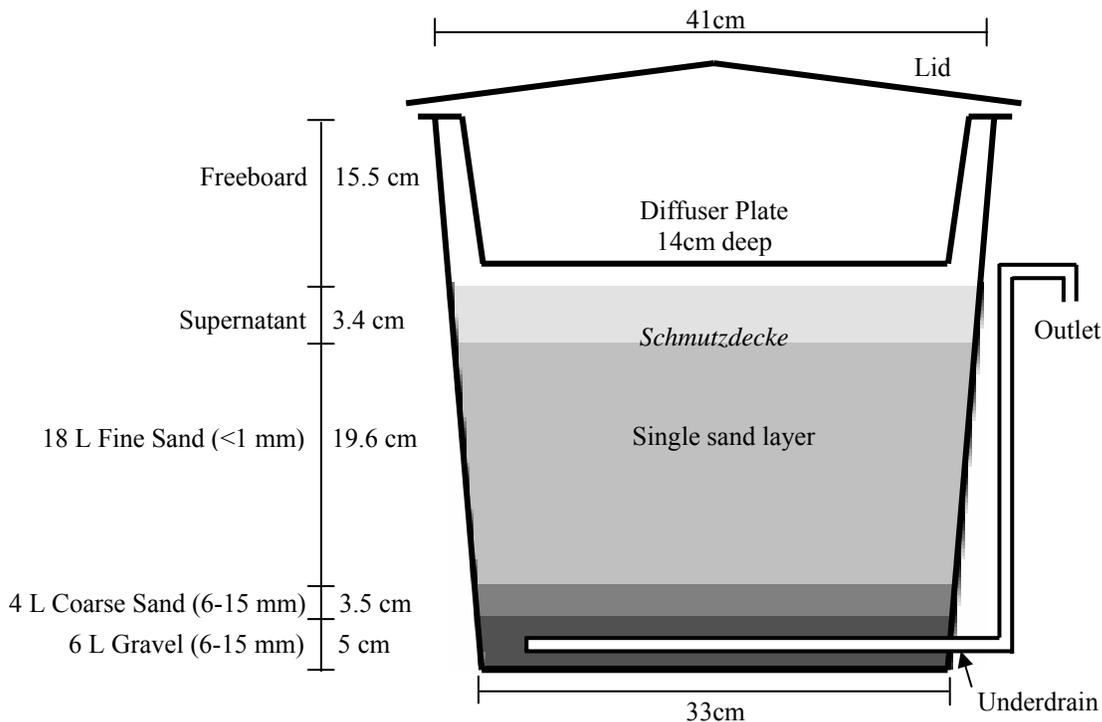
Figure 6-4 Single sand layer biosand filter (BSF A)
