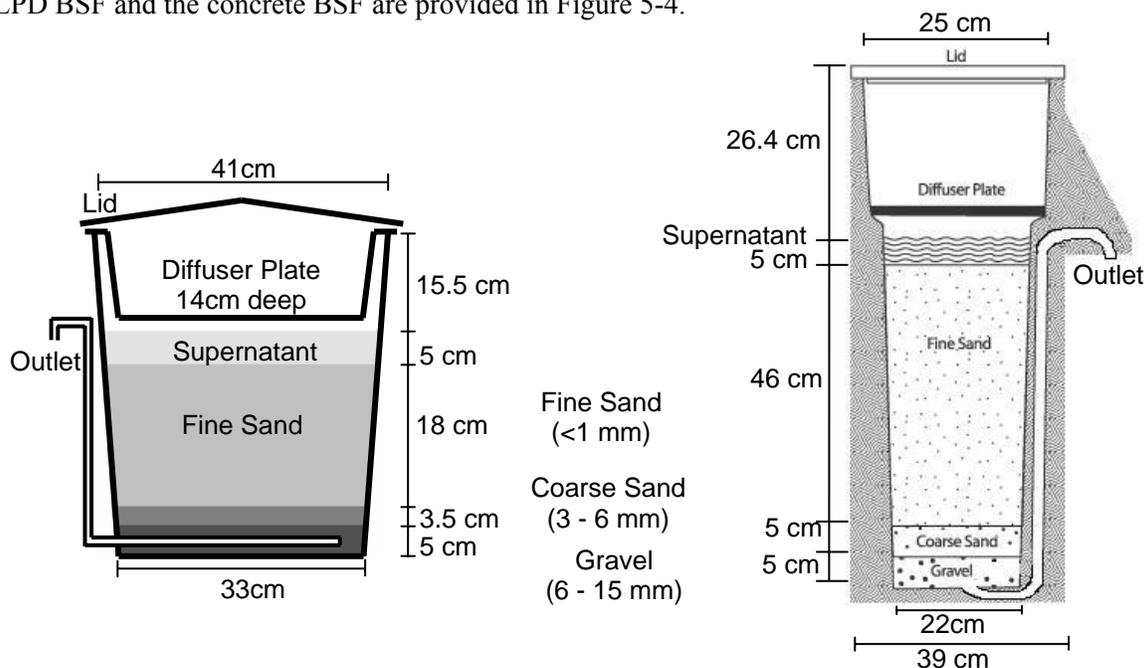
**Figure 5-4 Single sand layer biosand filters: a) local plastic design and b) concrete design**
