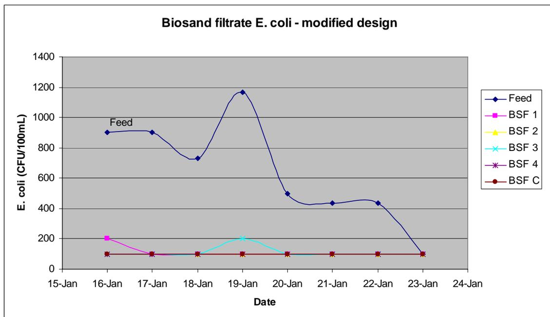
Figure 5-16 *E. coli* counts in BSF influent and effluent, modified operation
