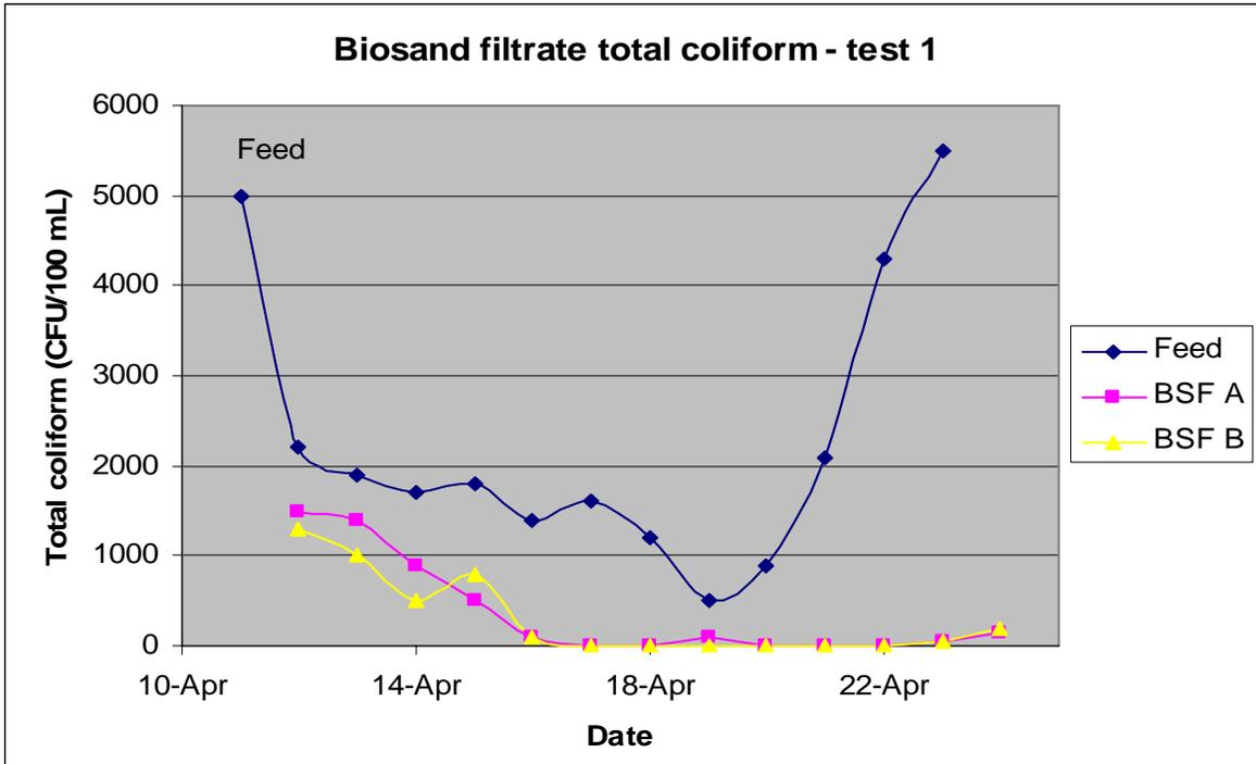
**Figure 6-10 Total coliform counts in BSF influent and effluent, test 1**
