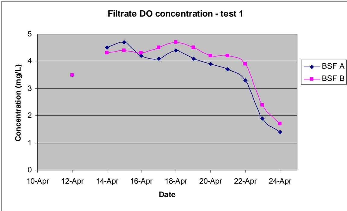
**Figure 6-12 Dissolved oxygen concentrations in the filtrate, test 1**
