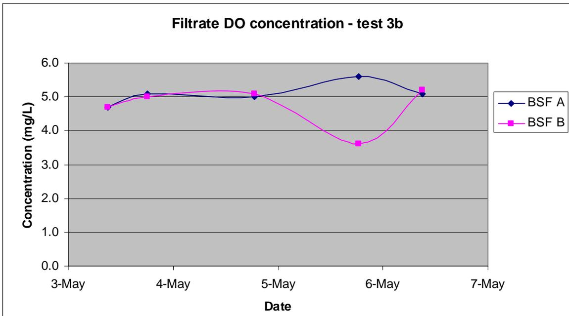
**Figure 6-27 Dissolved oxygen concentrations in the filtrate, test 3b**
