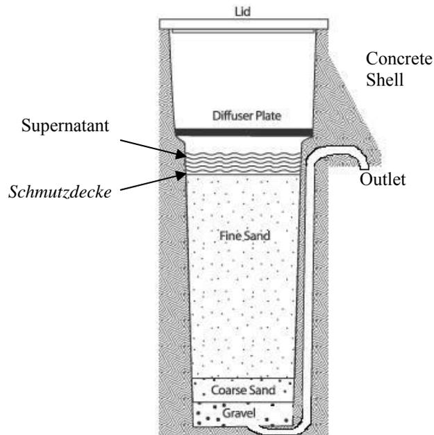
**Figure 3-4 CAWST style BSF filter layout**
