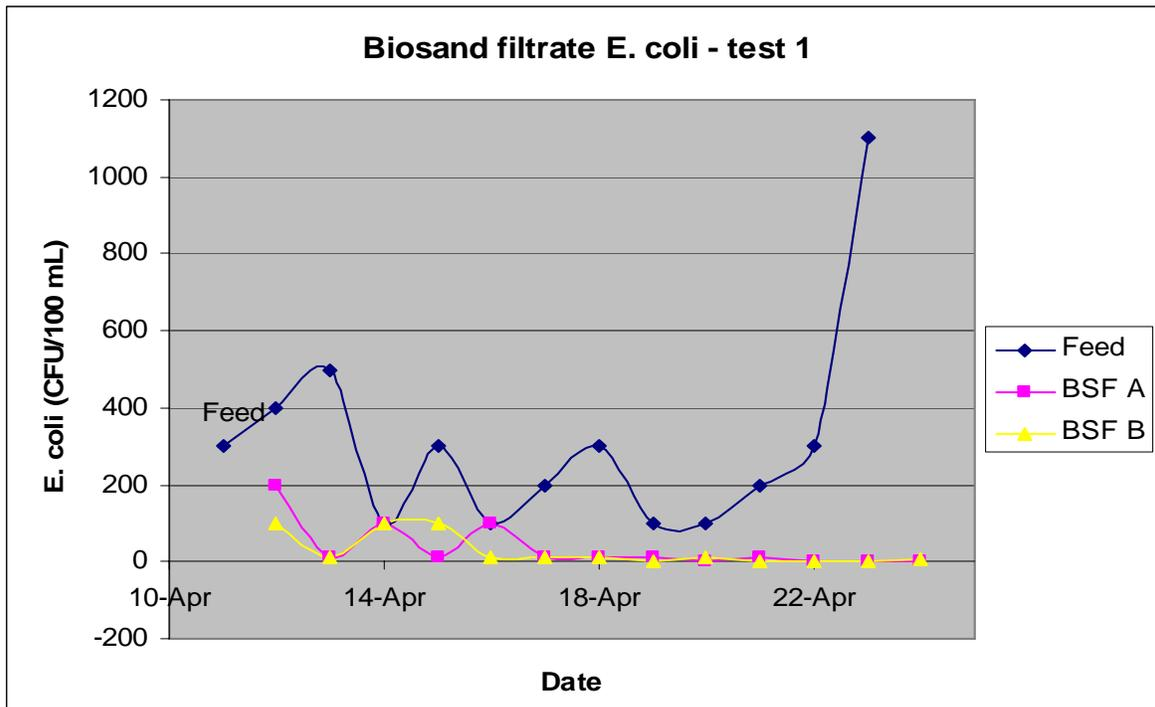
**Figure 6-9 *E. coli* counts in BSF influent and effluent, test 1**
