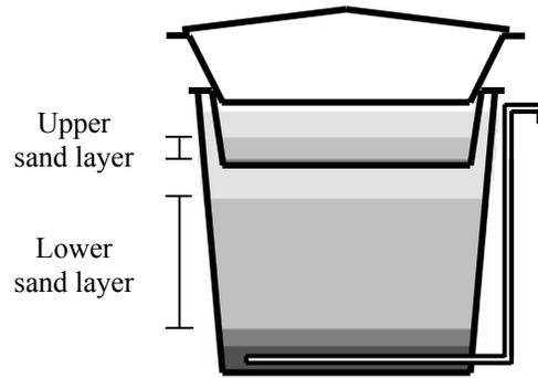
**Figure 6-1 Field test dual sand layer biosand filter**
