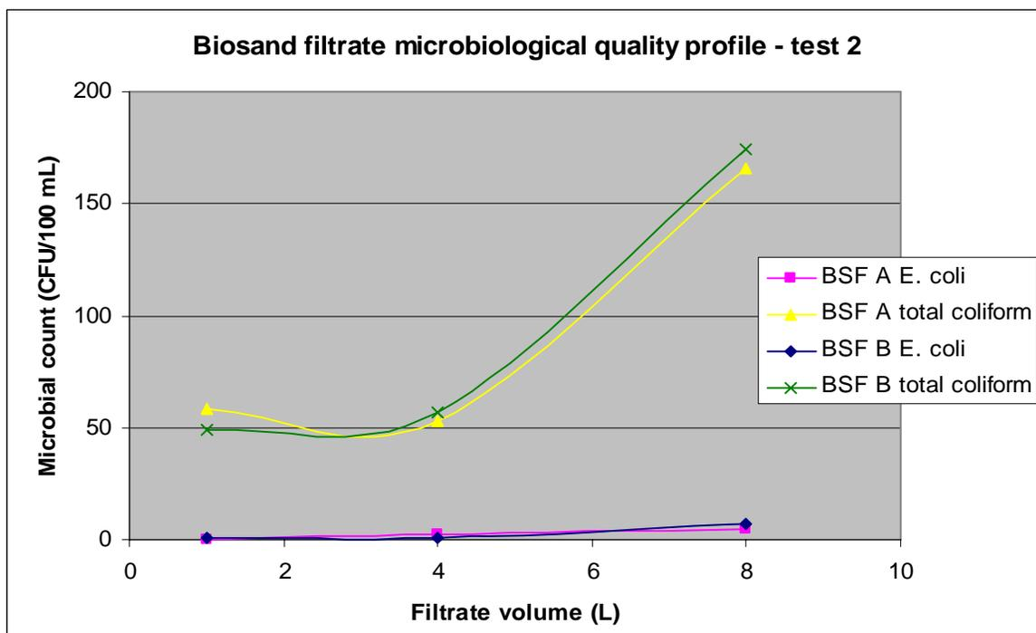
Figure 6-14 Effluent microbiological quality profile with filtrate volume
