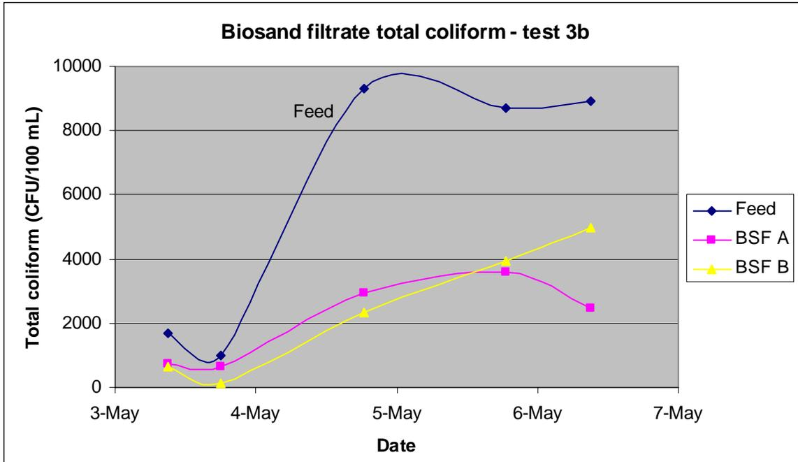
**Figure 6-26 Total coliform counts in BSF influent and effluent, test 3b**
