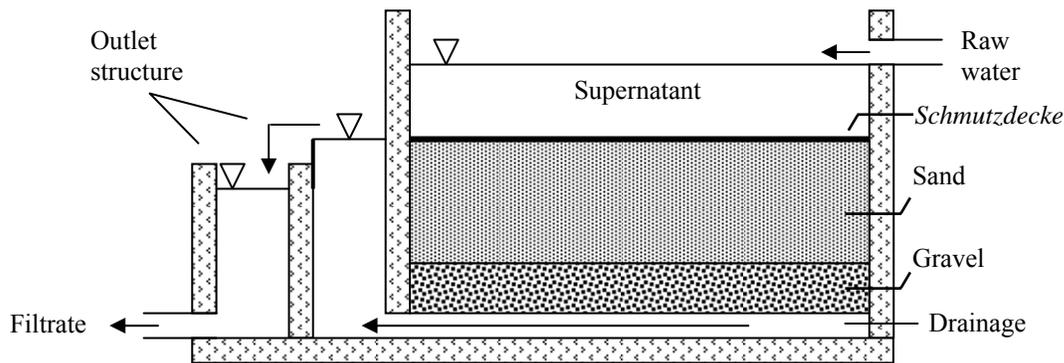
**Figure 3-1 Schematic layout of a slow sand filter**
