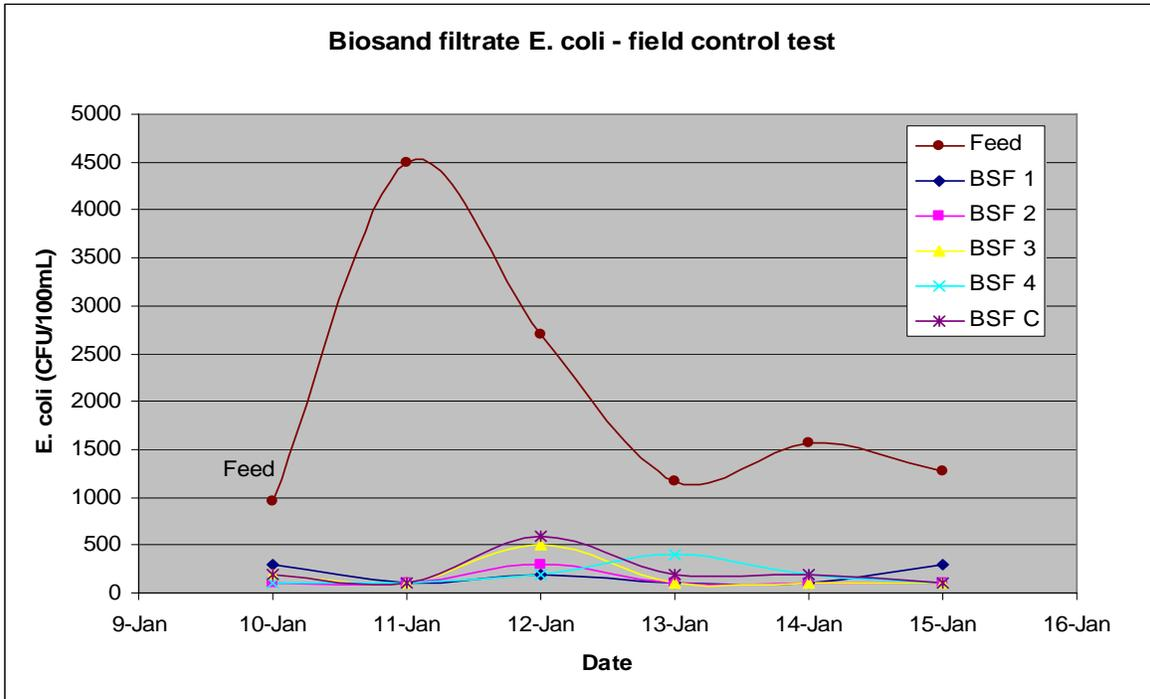
**Figure 5-13** *E. coli* counts in BSF influent and effluent, control tests
