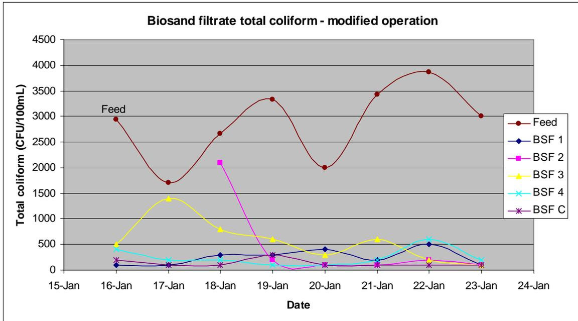
**Figure 5-17 Total coliform counts in BSF influent and effluent, modified operation**
