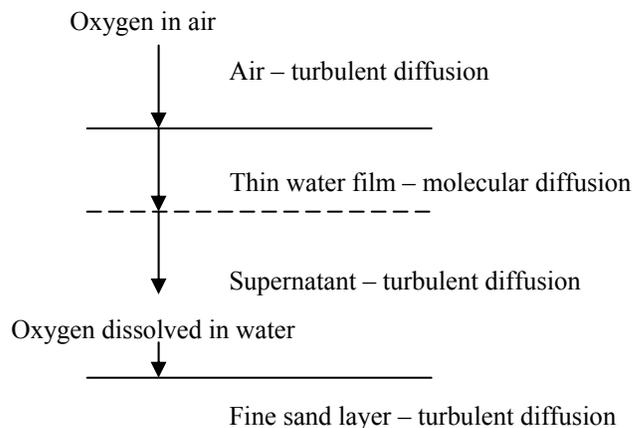
**Figure 6-2 Oxygen diffusion pathway in a single sand layer BSF**
