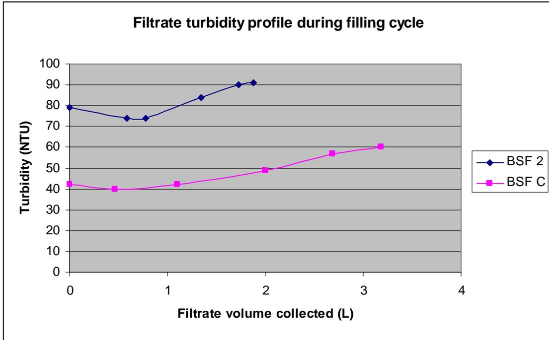
**Figure 5-10 BSF filtrate turbidity profile with filtrate volume**
