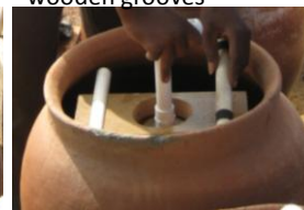
Inserting one than the other PVC arm into wooden grooves
