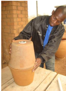
Rotating the two filters around to find the best alignment to minimize gaps between the two rims
