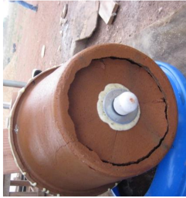
Figure 52 Bottom of KWK Cracked When Pressed Down Too Hard During Installation
