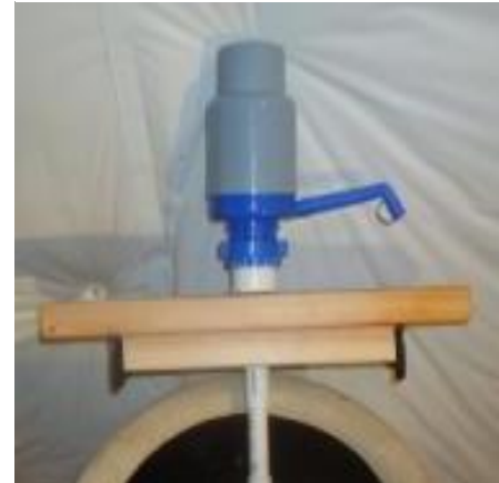
Figure 3 New design for wooden restraint to keep the KWK submerged Source: Chris Schulz
