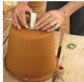
Gluing the steel washer to the ceramic filter, held in alignment by the PVC pipe
