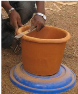
Filing the filter rims flat
