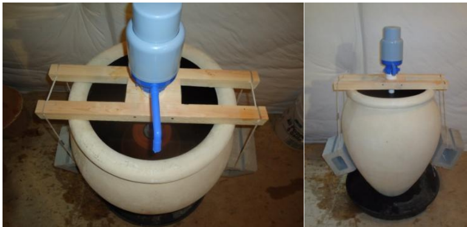
Figure 4 Another wooden restraint option for keeping the KWK submerged in the water vessel Source: Chris Schulz
