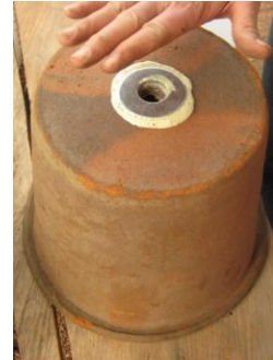
Figure 18 Metal Washer Sealed to the Ceramic Pot Filter Opening
