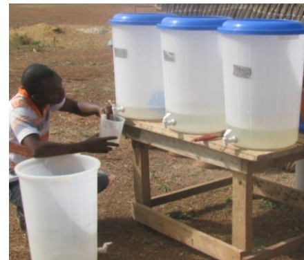
Figure 38 Measuring Volume Filtered by CPF
