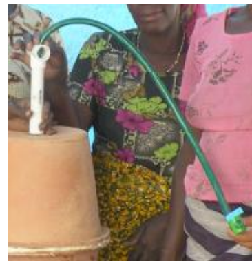
Figure 26 Tubing Used to Extract Water From the Top of the KWK Source: Espinoza 2010
