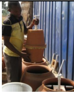
Picking up the KWK by the T-joint and putting it into water vessel
