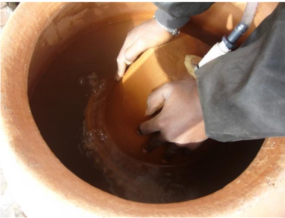
Figure 43 Leak Testing the Completed KWK
