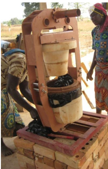
Figure 44 Pressing the CPFs in the Flowerpot-Shaped Hydraulic Press
