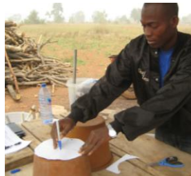
Marking off the center of the ceramic filter
