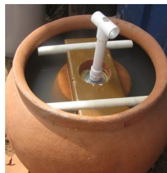
Figure 50 KWK Submerged with Wooden Restraint System
