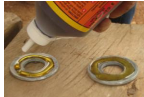
Applying glue to the washers
