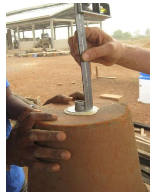
Figure 48 Measuring PVC Riser Pipe to Cut It for the KWK Height
