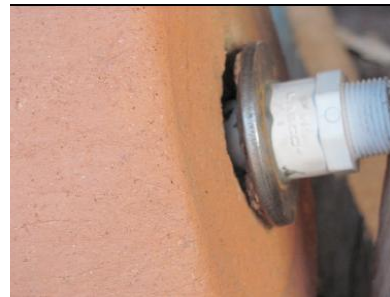
Figure 25 Ceramic Filter Breaking When Metal Washer is Attached With Epoxy Source: Espinoza 2010
