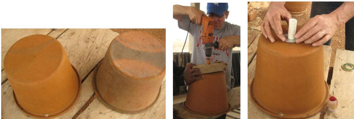
Figure 40 (left) Center Marked on CPFs (center) Hole Drilled Into Center of CPF (right) Metal Washer Sealed Around Hole
