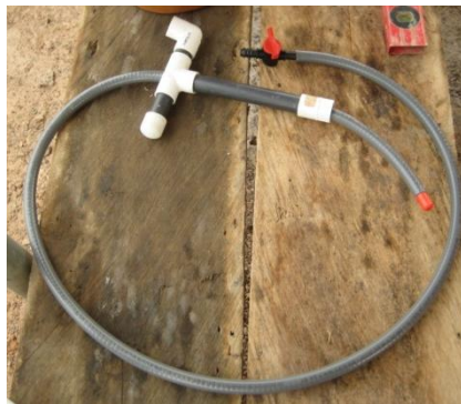
Figure 21 (left) Siphon Tube With Check Valve and Spigot Attached (right) Siphon Tube Installed in KWK
