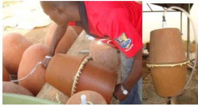
Replacing T-joint with rubber tubing
