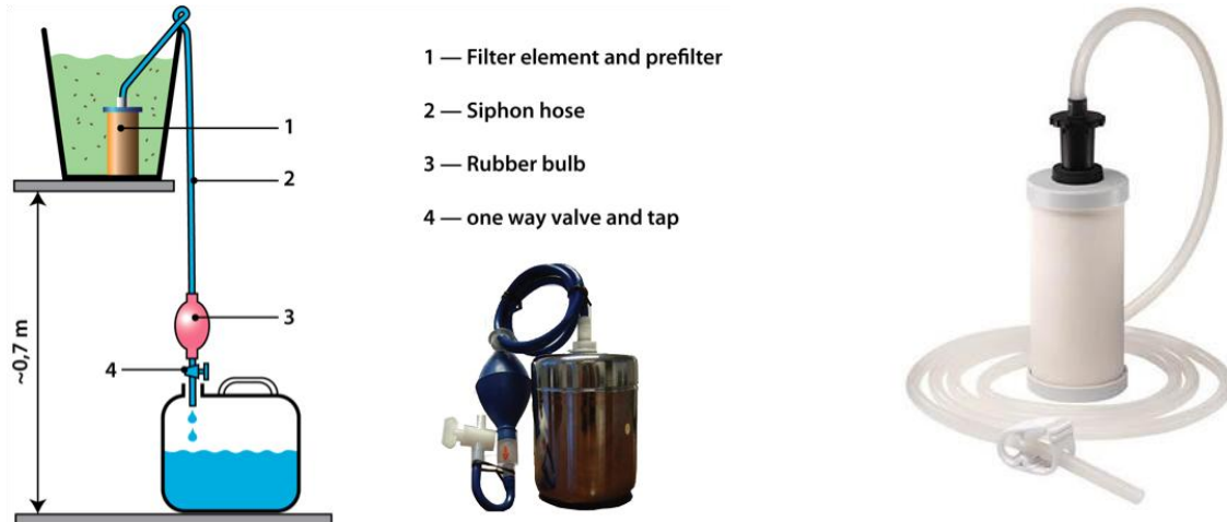
Figure 7 (a) Schematic of a Siphon Filter
