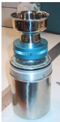
Figure 35 Membrane Filtration Field Unit
