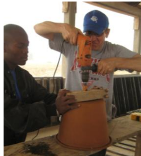
Drilling the hole with a wooden guide
