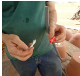
Applying superglue to check valve
