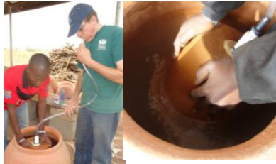
Re-applying glue to leaking spots
