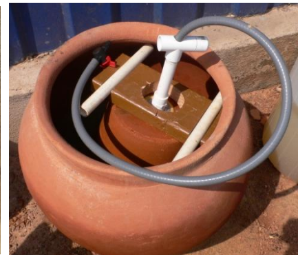
Figure 21 (left) Siphon Tube With Check Valve and Spigot Attached (right) Siphon Tube Installed in KWK
