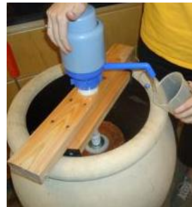
Figure 2 Water being removed from KWK with plastic hand pump
