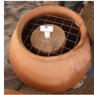
Figure 53 Wire Mesh Restraint System
