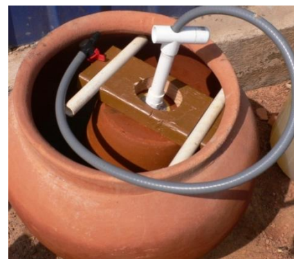
Figure 33 Wooden Restraint System Failing to Center KWK After KWK Fills With Water and Sinks
