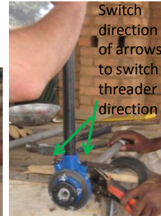
Threading the pipe – first by hand (left), and then using lever arm (right)
