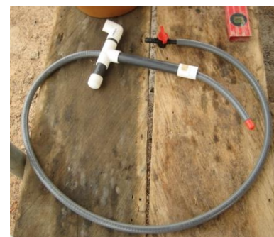
Figure 49 Siphon Threaded Through T-Joint
