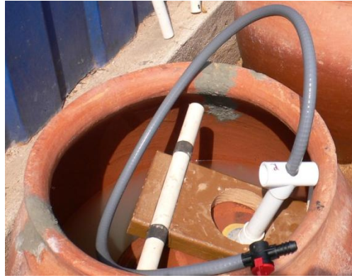
Figure 51 KWK Loose in Vessel After It Filled and Sank
