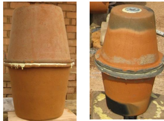
Figure 28 (left) Gorilla Glue to Seal KWK (right) SBR Bond to Seal KWK
