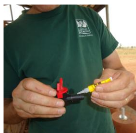
Applying superglue to shutoff valve
