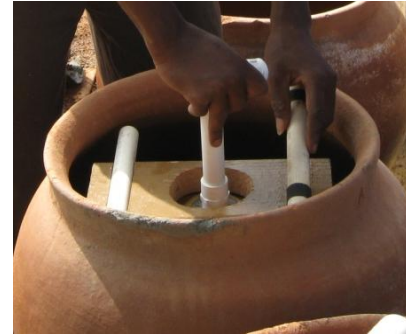
Figure 31 Wooden Restraint System to Submerge and Secure KWK
