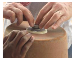
Pushing another O-ring onto the top of the PVC riser pipe
