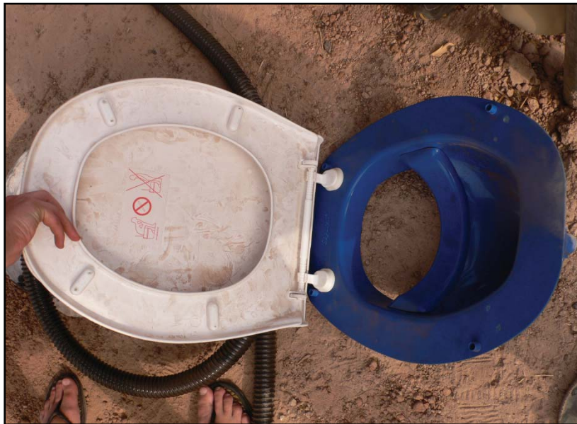
Figure 7-1 The type of urine-diverting seat used for the composting latrine
