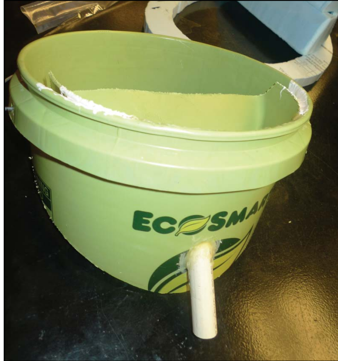
Figure 8-4 Prototype urine-separating toilet-seat using a bucket (side view) (Photo Credit: Mette Andersen)
