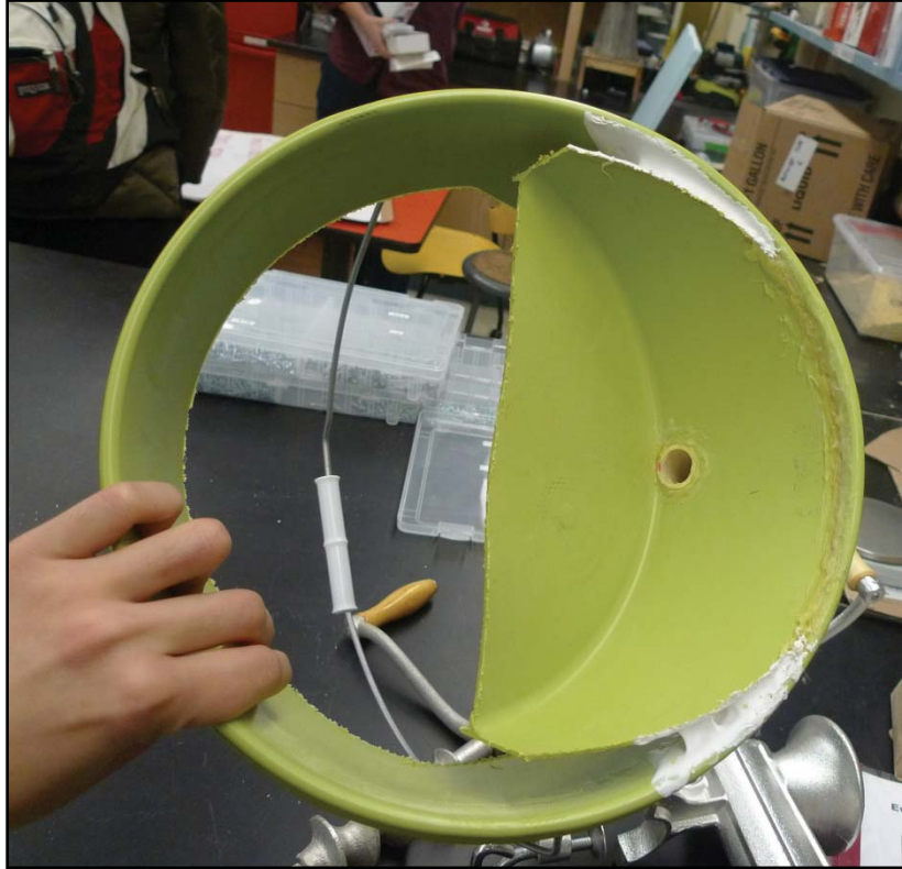
Figure 8-5 Prototype urine-separating toilet-seat using a bucket (top view) (Photo Credit: Mette Andersen)
