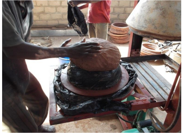
Figure 3-40: Abraham placing the clump of clay, rice husk "mixture" on the male mold
