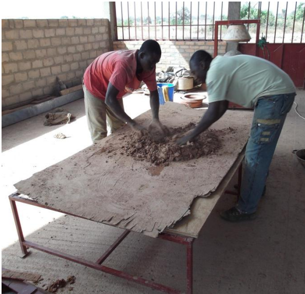
Figure 3-37: John and Alhassan mixing clay and rice husk
