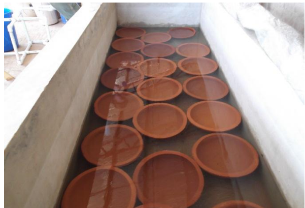
Figure 3-12: Soak Tank with Filters
