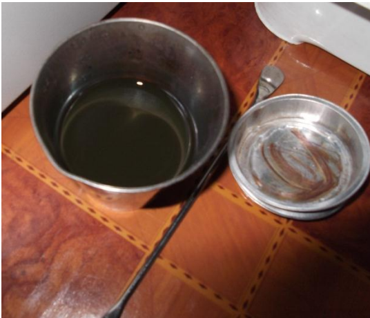
Figure 3-28: Stock solution, spatula, and metal weighing dish used for creating colloidal silver application solution
