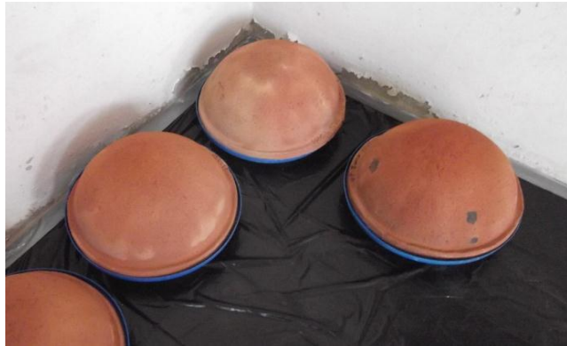
Figure 3-32: Newly painted CPFs drying
