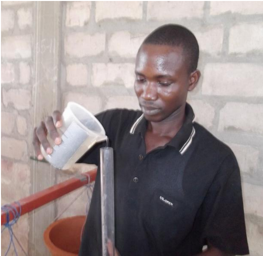
Figure 3-7: Karim pours sample into turbidity tube
