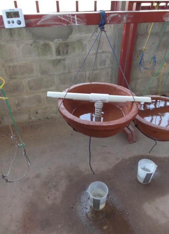
Figure 3-17: Flow Rate Test (both the collection method and T-device method are shown)
