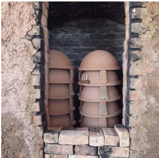
Figure 3-44: CPFs stacked eight high in the kiln
