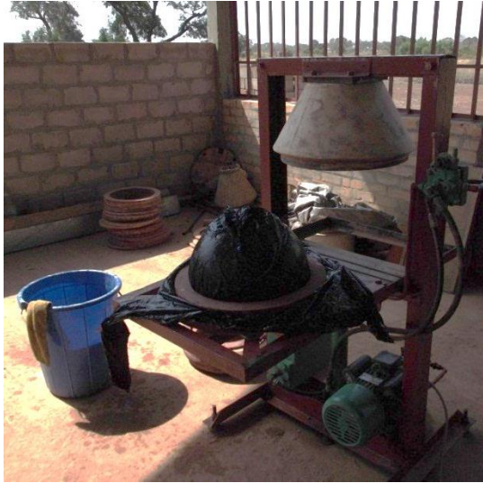
Figure 3-39: The hemispheric hydraulic press with plastic bag and wooden annulus
