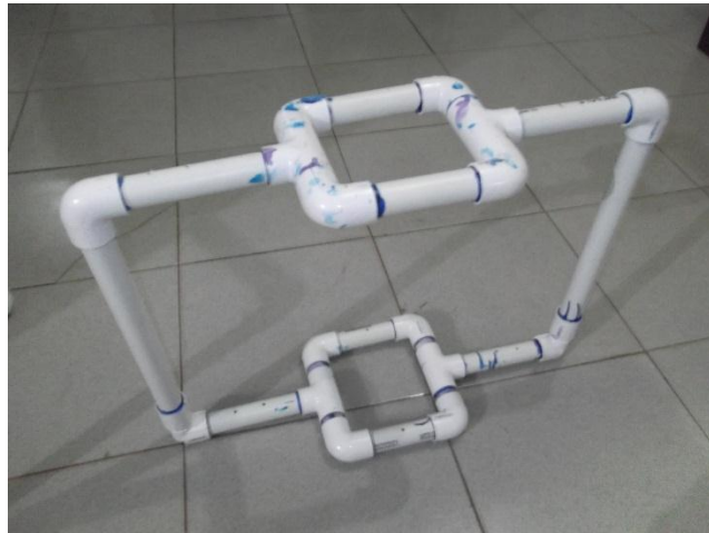
Figure 3-14: PVC Pipe "Basket" for Apparent Porosity Test
