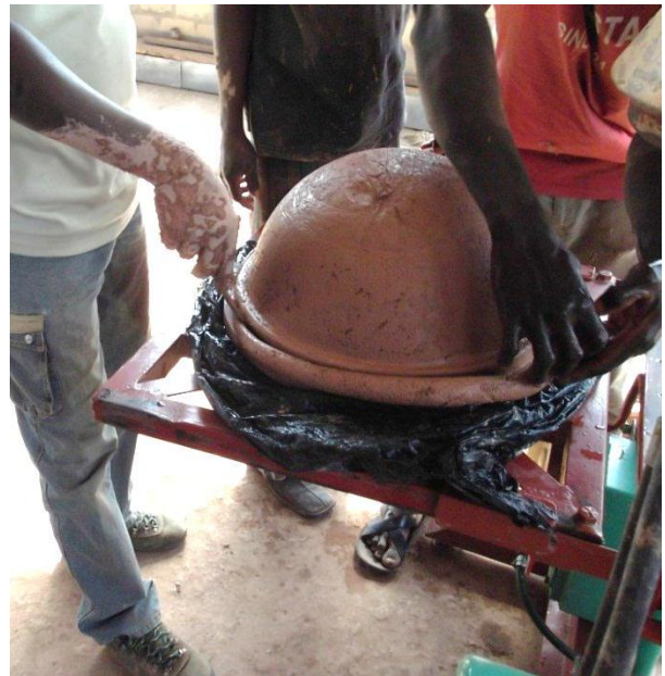
Figure 3-42: John and Alhassan removing the excess clay from the CPF
