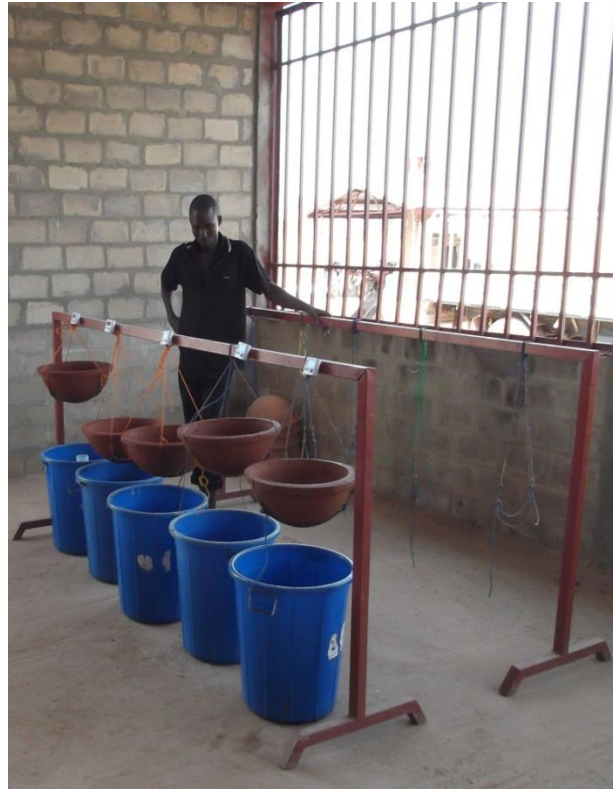
Figure 3-18: Flow Rate Test Setup with metal racks
