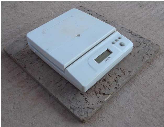
Figure 3-11: Cen-Tech 70 Lb/32 Kg Digital Postal Scale on plywood and concrete surface
