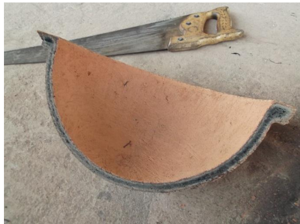
Figure 3-27: A CPF cut in half by saw
