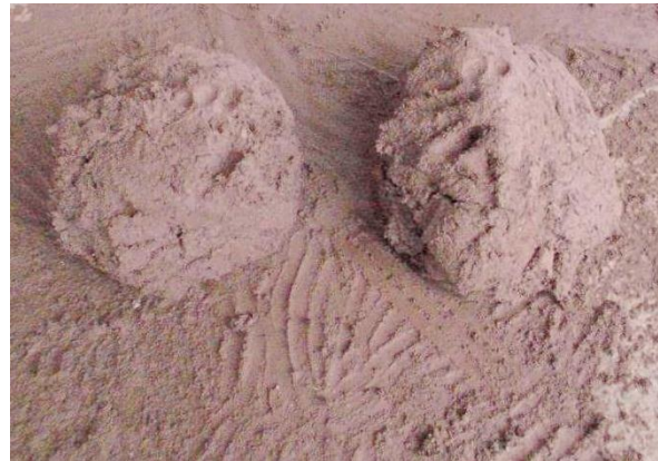
Figure 3-38: Clumps of clay, rice husk, and water ready to be pressed
