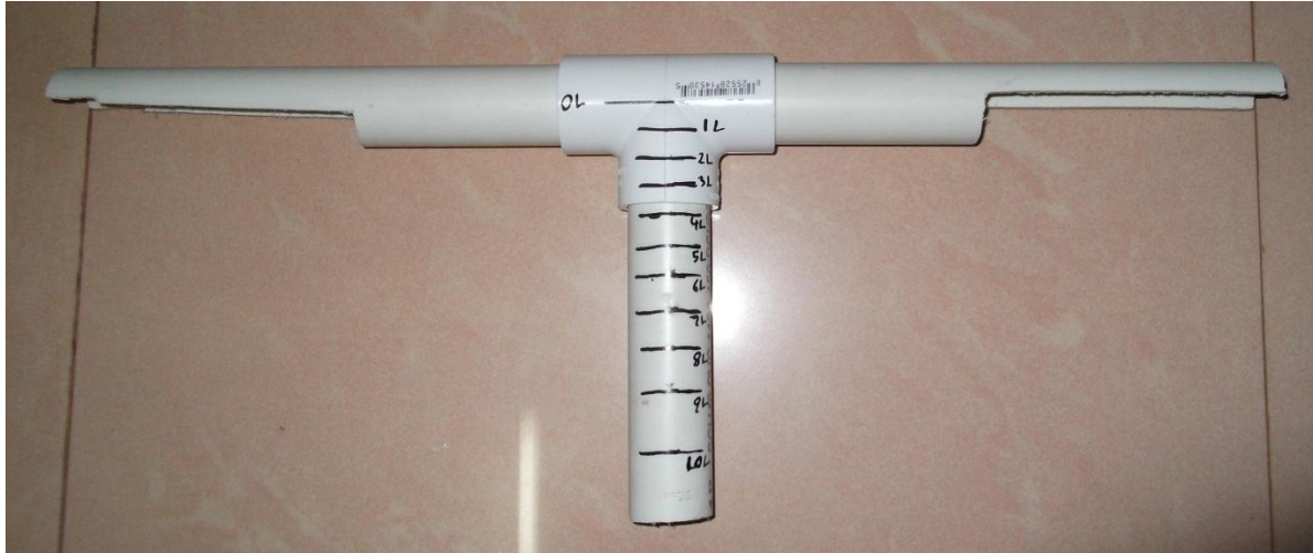
Figure 3-20: T-Device for the Hemispheric CPF
