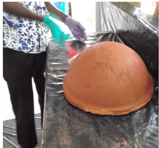
Figure 3-31: Karim painting a CPF with colloidal silver
