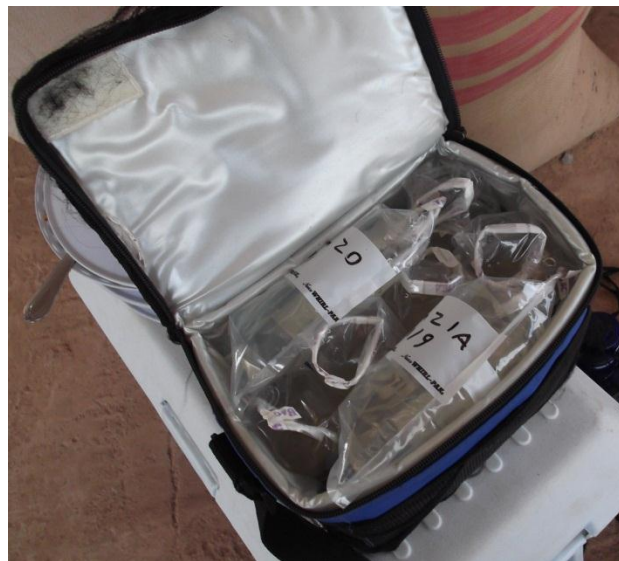
Figure 3-26: Cooling and storage of filtrate samples before taking back to the lab for testing
