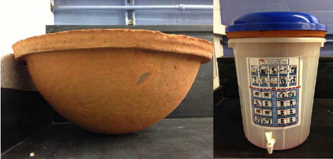
Figure 1-1: Hemispheric ceramic filter element (left) and complete unit (right)
