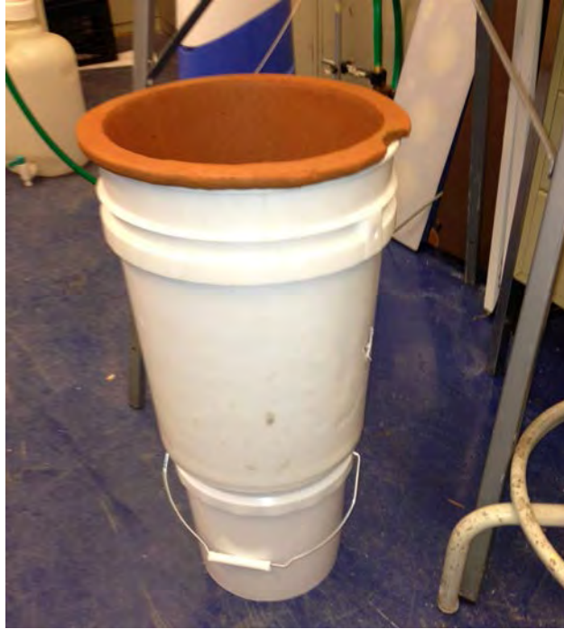
Figure 2-2: Lab testing of flowerpot filter
