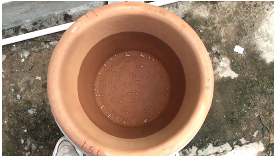
Figure 5-21: Droplets appearing on the inside surface of the filter.
