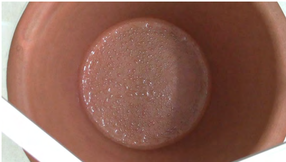
Figure 5-22: Droplets appearing on the inside surface of a second filter. This filter has a higher density of distinct droplets indicating a different internal structure.
