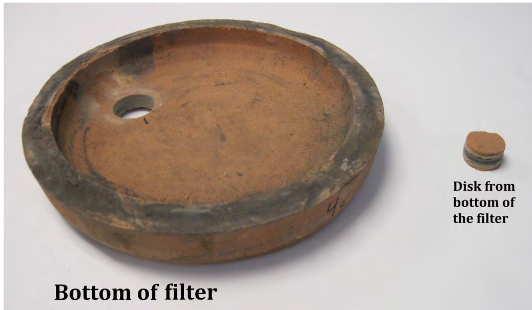
Figure 3-1: Disk cut from the bottom of the filter. The disk is used in the experiments.
