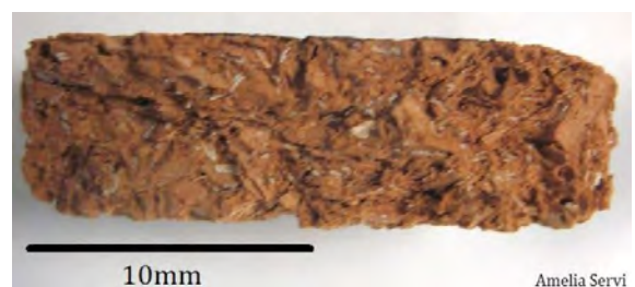
Figure 3-8: Inside surface of a disk produced with risk husk sieved to 710-850 \mu\text{m} .
