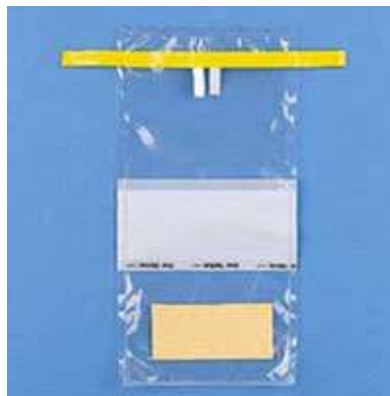
Figure 12: Example of Whirl-Pak® sampling bag used to collect water samples (LabShop).
