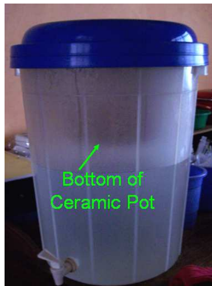
Figure 20: Point to which ceramic pot extends into storage receptacle.
