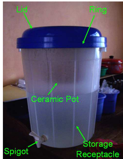
Figure 5: The Kosim Filter and its components (PFP, 2007).
