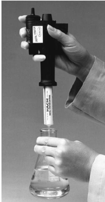
Figure 17: Hach Digital Titrator assembly (Hach, 2006).
