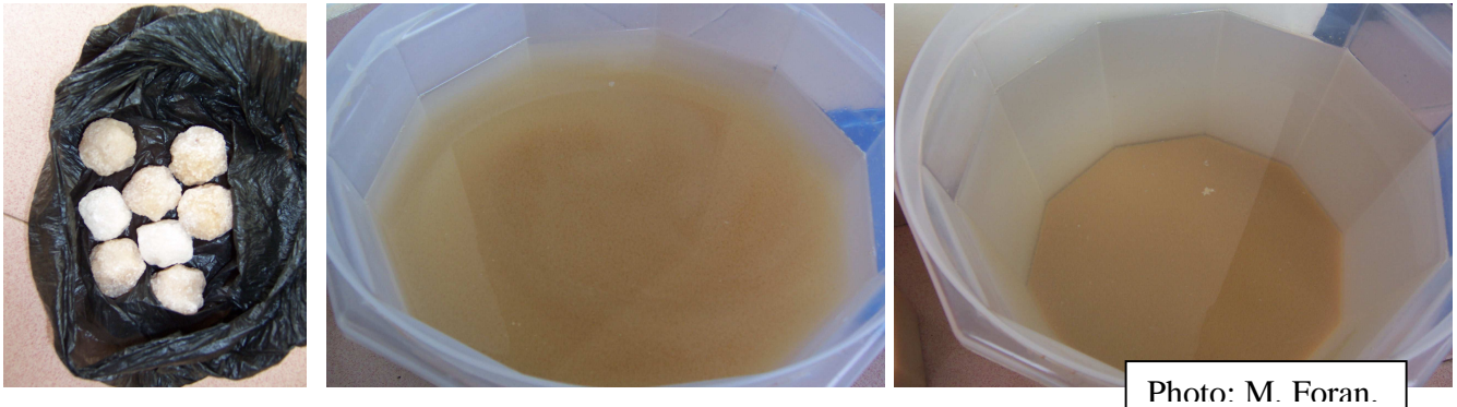
Fig. 1 alum balls; Fig 2 turbid surface water from “dugout”; Fig. 3 after alum coagulant.
