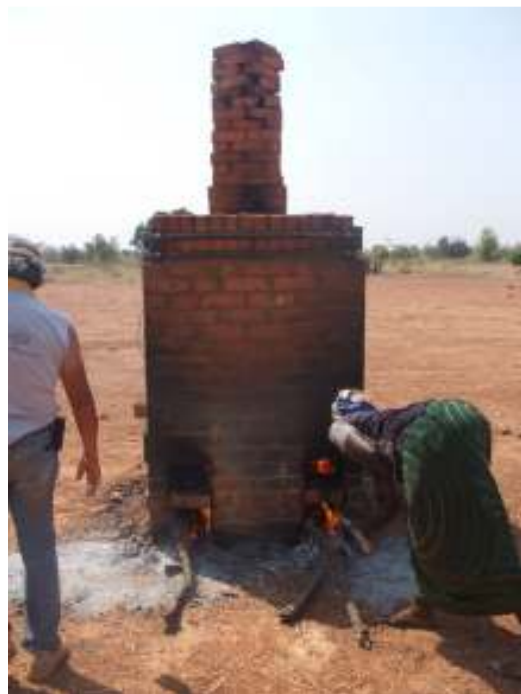
Figure 4-6: Downdraft Mani Kiln, Showing Fireboxes
