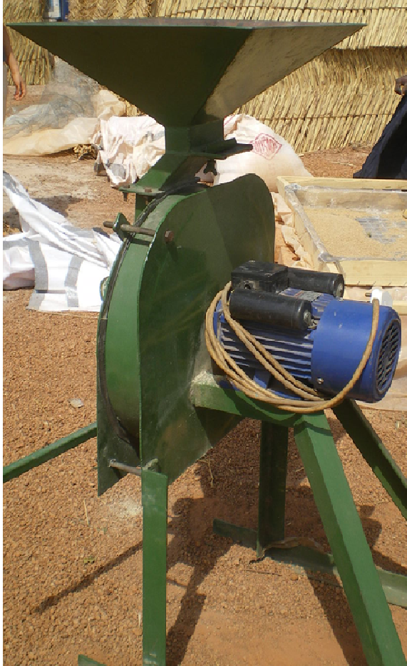
Figure 4-2: Hammermill (Closed at Left, Photo Credit: Leah Nation, 2010; Open at Right)
