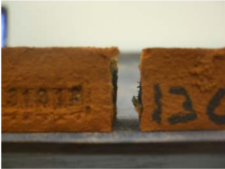
Figure 5-10: Vertical Failure Plane Exhibited by Sample 13G
