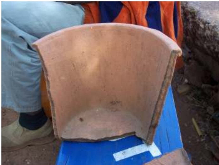
Figure 2-2: Ghanaian Filter with Presumed Impact Breakage (Murcott, 2009)
