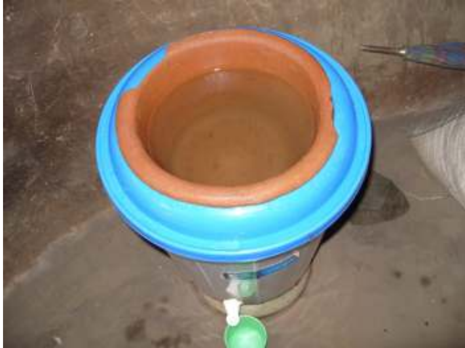
Figure 2-1: Ghanaian Filter with Broken Lip (Murcott, 2009)
