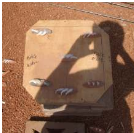
Figure 5-7: Schematic of Kiln Loading (Left) and Photograph of Pyrometric Cones Taken After Firing with Relative Positions Preserved (Right) (Watters 2010)
