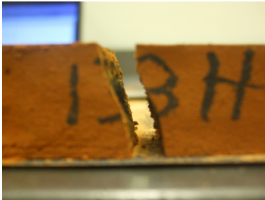
Figure 5-11: Angled Failure Plane Exhibited by Sample 13H
