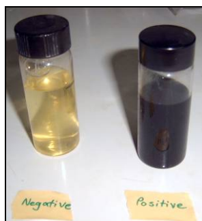
Figure 6: Negative (yellow) and Positive (black) results for H 2 S bacterial water testing
