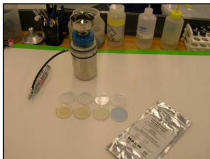
Figure 7: Membrane Filtration Testing Materials
