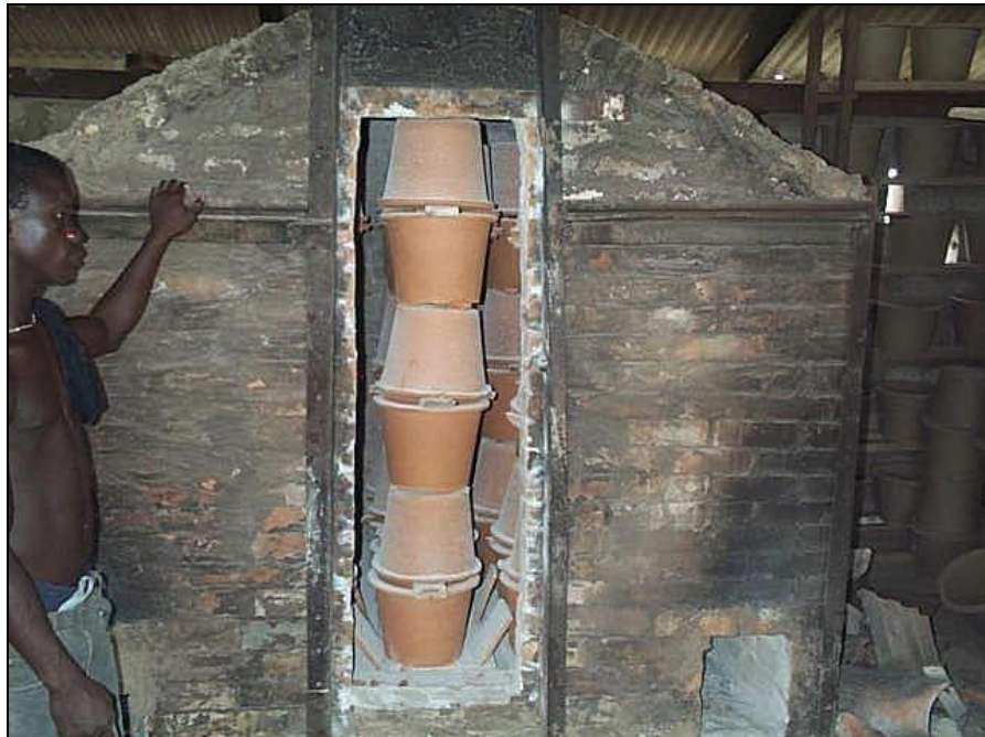
Figure 7: Kiln for firing ceramic filters in Accra, Ghana. Photo Credit: Ron Rivera
