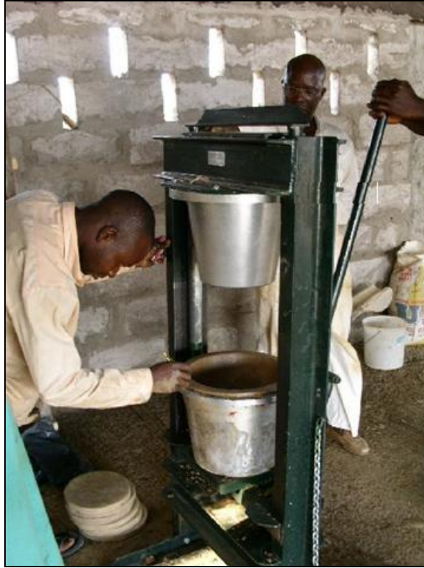
Figure 6: Hydraulic press used to make the filter in Accra, Ghana. Photo Credit: Ron Rivera
