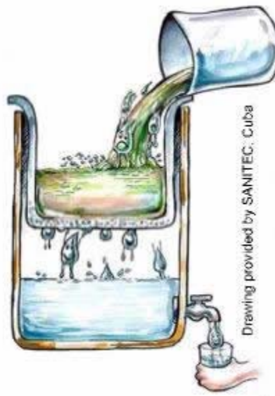
Figure 5: Diagram of the Filtron system (PFP 2007). Water passes through a clay filter at the top into a lower storage receptacle. The spigot allows users to access the filtered water.
