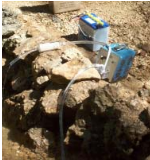
Figure 5-1: Filtering Haitian Water: Generator pumps water from source through Gelman filter, and returns water to the source downstream of uptake
