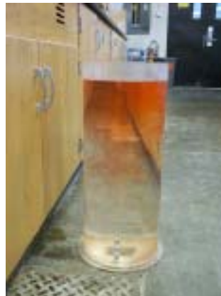
Figure 19 Mixing of 1 ml of bleach in a stratified water column.
