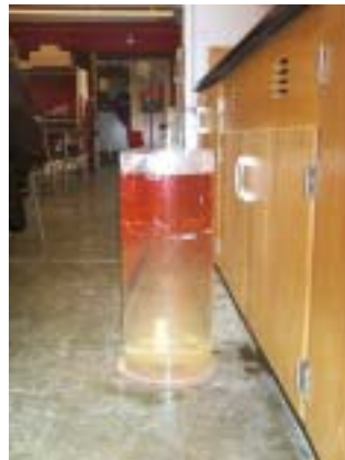
Figure 12 Artificial stratification. Hotter and therefore less dense water is red in color.
