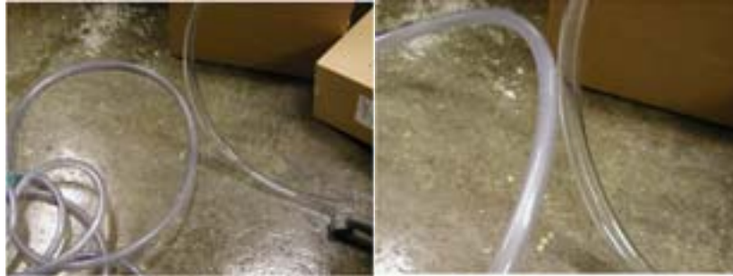
Figures 5.2 a and b: A comparison of the PVC tube used for Spirasol system experiments in Cambridge (left) and an unused PVC tube kept mostly in darkness (right). A) From afar, one can see the bluish tint beginning to develop. B) A close-up shot shows that the Spirasol tube has become rather opaque over the course of a month.
