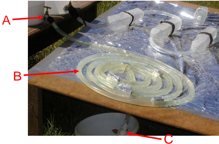
Figure 3.1: Constructed prototype of the Spirasol system. A) Three-quarter-inch faucet; B) Three-quarter-inch inner-diameter PVC tube; C) Three-quarter-inch PVC ball valve.
