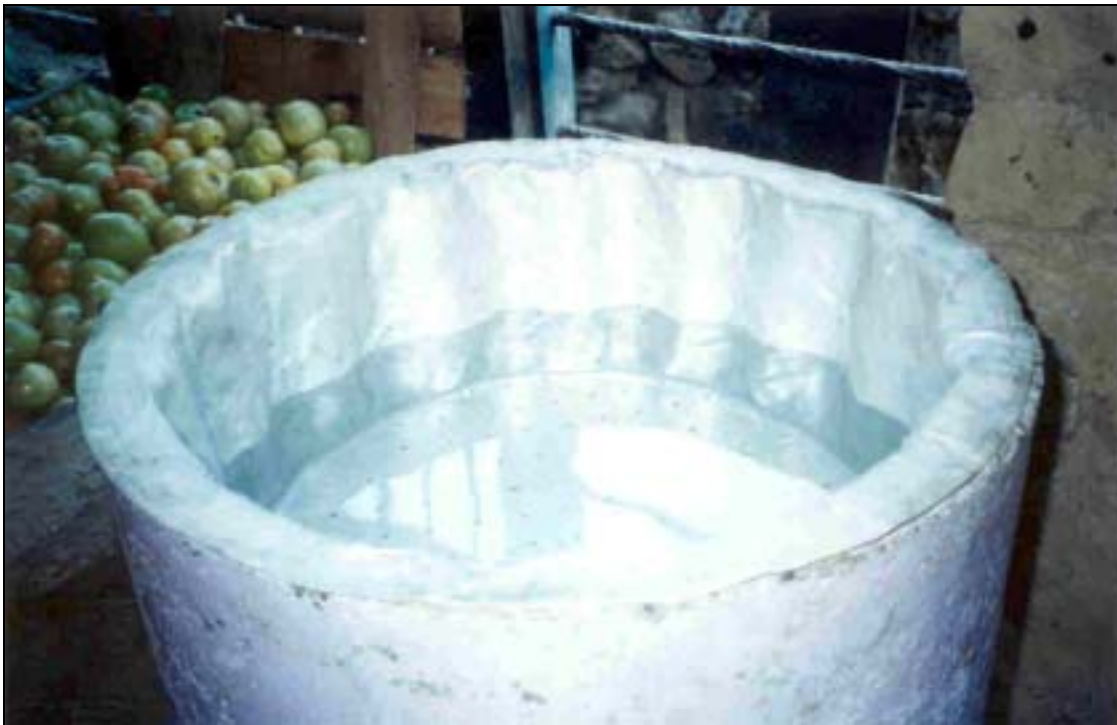
Figure 19: A metal pot used as a diffuser basin in a round BSF
