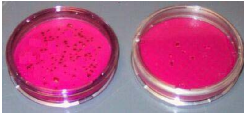
Figure 39: Membrane filtration total coliform results - Charles River water before filtration (left); after filtration (right)
