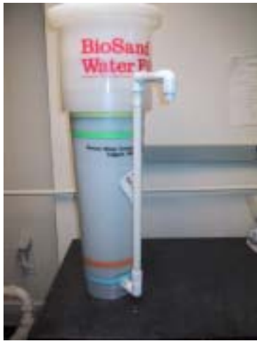
Figure 4: Plastic BSF from Davnor Water Treatment Technologies Ltd.
