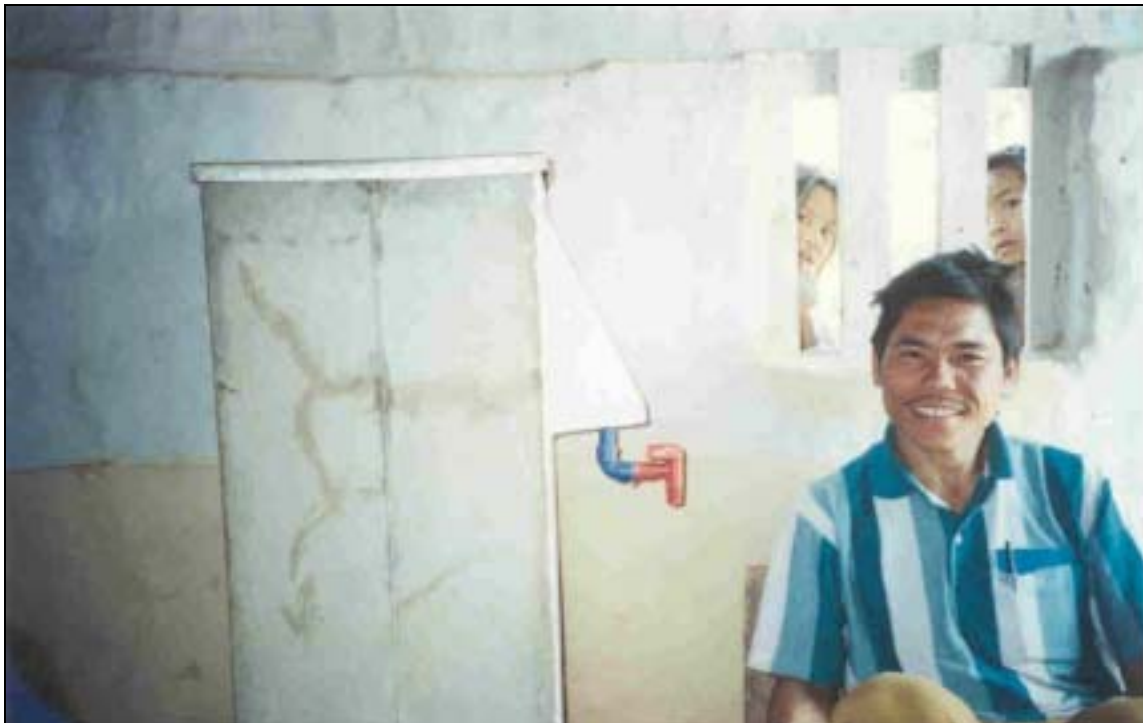
Figure 38: A cracked BSF that was mended by a technician
