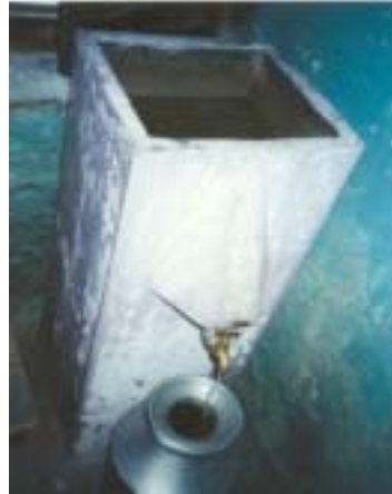
Figure 5: Concrete BSF made from shop drawings provided by Davnor Water Treatment Technologies Ltd.
