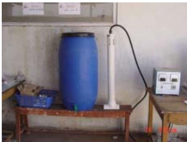
Figure 3.1: Sodium Hypochlorite Generator in Kathmandu, Nepal (Morganti, 2002)
