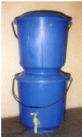
Figure 4.4: Modified-Bucket Chlorination System, with Candle Filter
