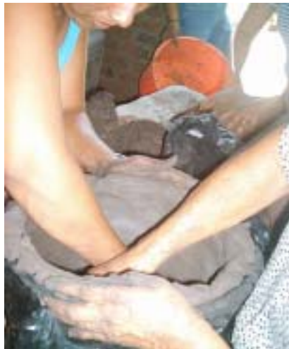
Figure 2-7 Step 6. Participants cover inside surface of mold with strips of clay
