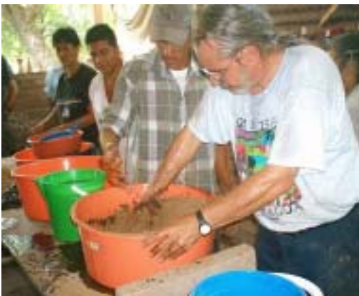
Figure 2-5 Step 3. Ron sprinkles clay and mixes with sawdust
