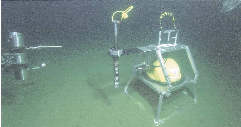
Fig. 2. Experimental apparatus on the seafloor as recorded by the HDTV video camera on the ROV Ventana . At the right is the time-lapse camera system with the sample rack containing the four hydrate samples. At the left is the open pressure vessel with release valve and differential pressure gage, secured by one of the ROV's two robotic arms. The other arm is just visible at the upper right.
