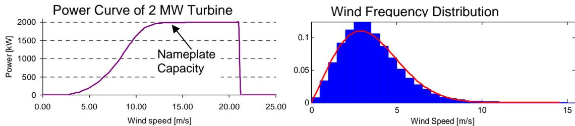
**Figure 2.2** Typical wind turbine power curve (left panel) and the statistics of wind variability (right panel) given by a histogram and Weibull probability density fit.
