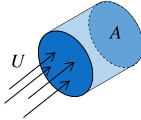
**Figure 2.1** Schematics of air flow at velocity  $U$  through area  $A$ . The cylinder depicts the volume flowing in unit time  $dt$  through area  $A$ .
