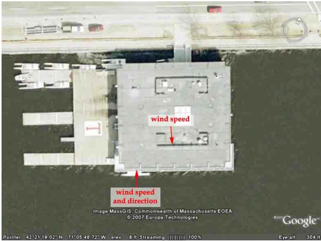
Figure 20. W8 Anemometer locations 48 .
