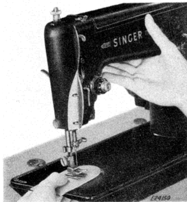
Fig. 35. Changing the Throat Plate
