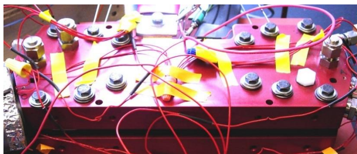
Figure 7 Assembled fuel cell with an active area of 50 cm 2 .
