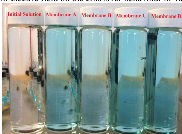
(b) The effect of membrane characteristics on the crossover behaviour of vanadium species
