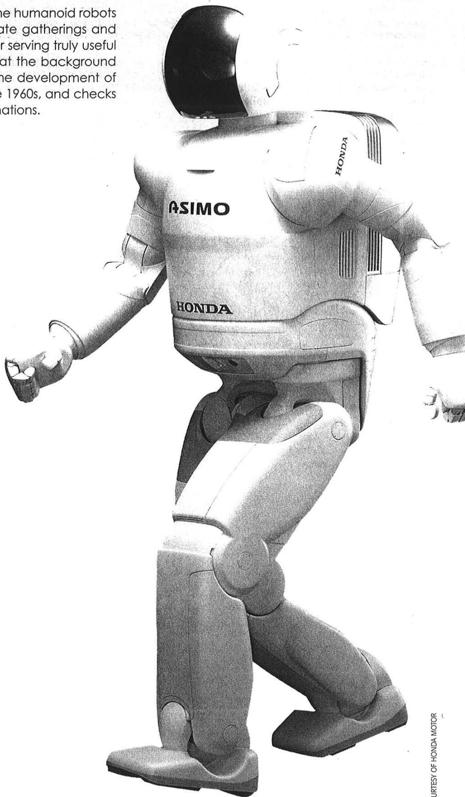
Honda's ASIMO spearheads the company's near-future vision of "one robot for each household." ASIMO is 120 centimeters tall—about the optimum height for household applications—and weighs 43 kilograms.
