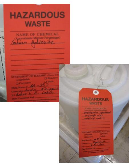
Finding 4 44505: SAA-4: Tags or labels on chemical waste containers were missing, incomplete, inaccurate or not legible. (Satellite Accumulation Area (SAA))
