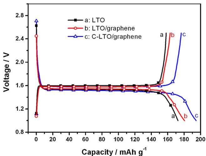
Fig. 3. Galvanostatic charge–discharge curves of LTO, LTO/graphene, C-LTO/graphene samples at 0.2C charge–discharge rate.
