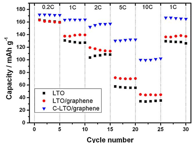
**Fig. 4.** Reversible capacity of LTO, LTO/graphene and C-LTO/graphene products at different charge-discharge rates.
