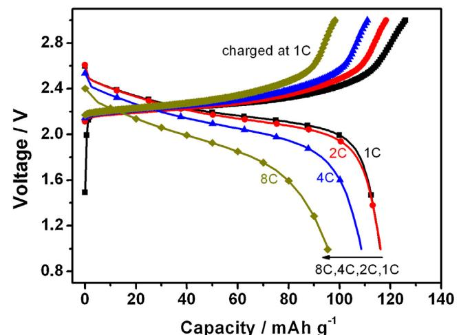
**Fig. 8.** Charge and discharge curves of the full-cell consisting of the C-LTO/graphene negative electrode and the  $\text{LiNi}_{1/3}\text{Co}_{1/3}\text{Mn}_{1/3}\text{O}_2$  positive electrode at different discharge rates.
