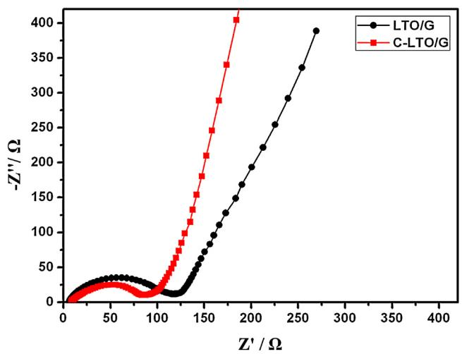
**Fig. 6.** AC impedance spectra of LTO/graphene and C-LTO/graphene at the state of full charged.
