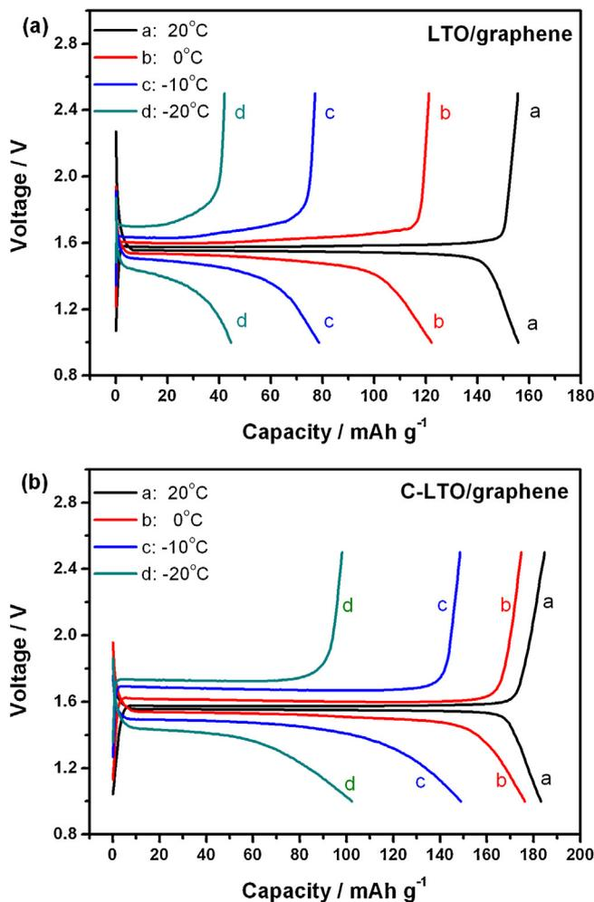
Fig. 7. Discharge and charge curves of (a) LTO/graphene and (b) C-LTO/graphene anode at 0.2 C rate at various temperatures.
