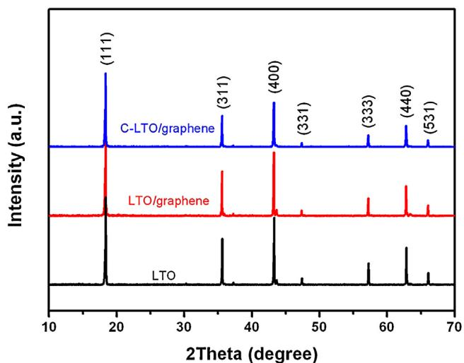
Fig. 1. XRD patterns of purified LTO, LTO/graphene composite and C-LTO/graphene composite.
