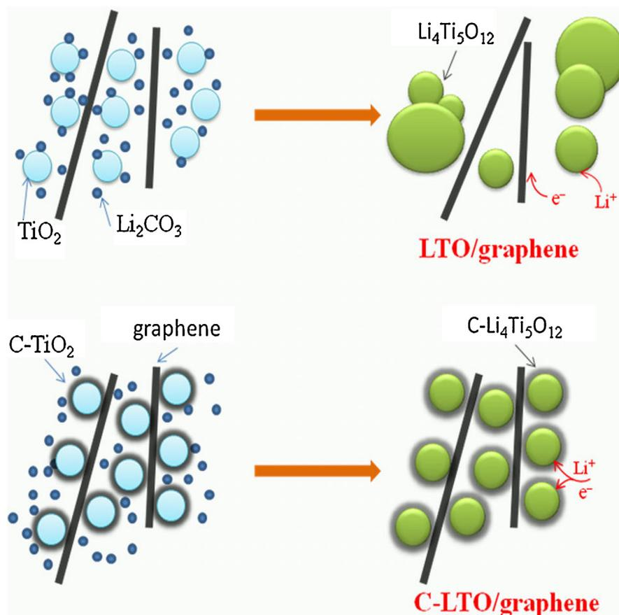
**Fig. 9.** Schematic illustration of the effects of carbon coating in LTO/graphene composites.
