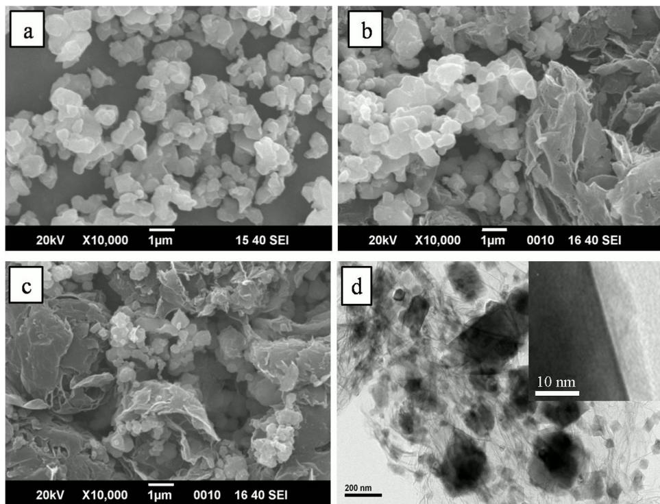
**Fig. 2.** SEM images of (a) LTO, (b) LTO/graphene, (c) C-LTO/graphene and TEM image (d) of C-LTO/graphene.
