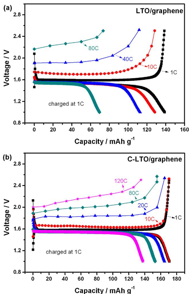
Fig. 5. Charge and discharge curves of (a) LTO/graphene and (b) C-LTO/graphene samples that discharge at 1 C and charged at different rates.
