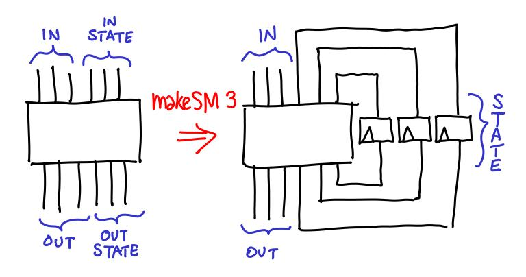
Here is an extended example of how you might use the API. Consider a purely combinational circuit that simulates state through a number of input and output ports. We'd like to hook those ports up to latches, so our circuit is intrinsically stateful.
