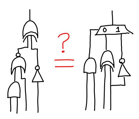
What does it mean to verify a circuit? If we are optimizing a circuit, we would like to make sure each optimized version is equivalent to the original version. So verification is equivalence checking.
