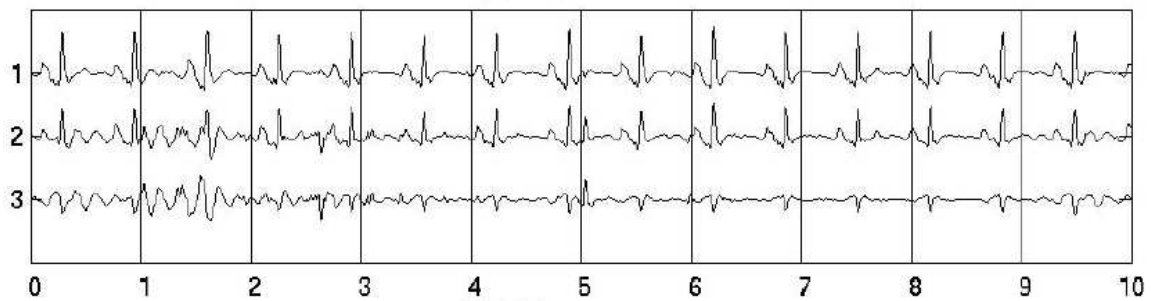
Figure 1: 10 seconds of 3 Channel ECG. Note the high amplitude movement artifact in the first two seconds and the 10 th second. Note also the QRS-like artifacts around 2.6 and 5.1 seconds
