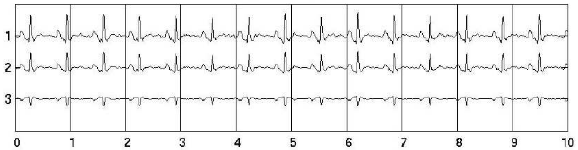
Figure 8: 10 seconds of data (from Fig. 1) after ICA decomposition, (see Fig 7) and reconstruction with noise channels set to zero.
