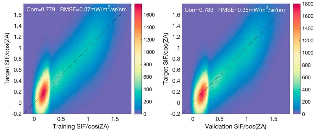
**Figure 1.** Performance of the neural network retrieval of Global Ozone Monitoring Experiment-2 SIF normalized by the cosine of Sun solar zenith angle using first four Moderate Resolution Imaging Spectroradiometer reflectance channels, at 0.5°, 16-day resolution over the training and validation test. The density of scatter points is represented by the shading color. The diagonal black dashed line depicts the 1:1 relationship.
