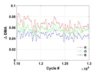
Figure 5. DMA parameter evolution over cycles in a GSST device with 180 nm thick GSST and 740 nm thick SiN<sub>x</sub> encapsulation.
