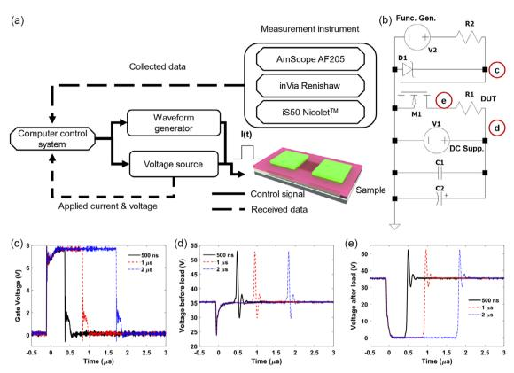
Figure 2. a) Block diagram of the multifunctional characterization platform. b) Electric circuit diagram for high voltage pulse generation. c—e) Voltage measurements from an oscilloscope across the load measured at the transistor gate; d) before the load; and e) after the load.
