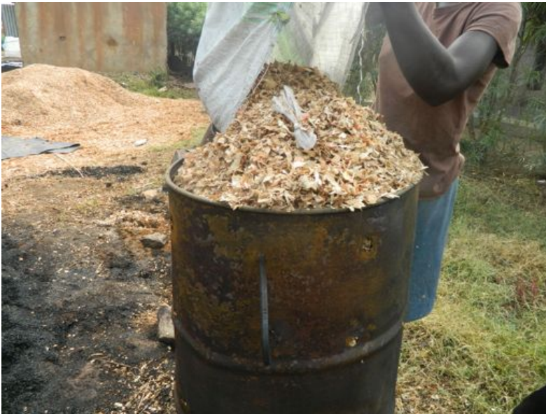
2. The ground husks and saw dust poured into kiln for carbonizing
