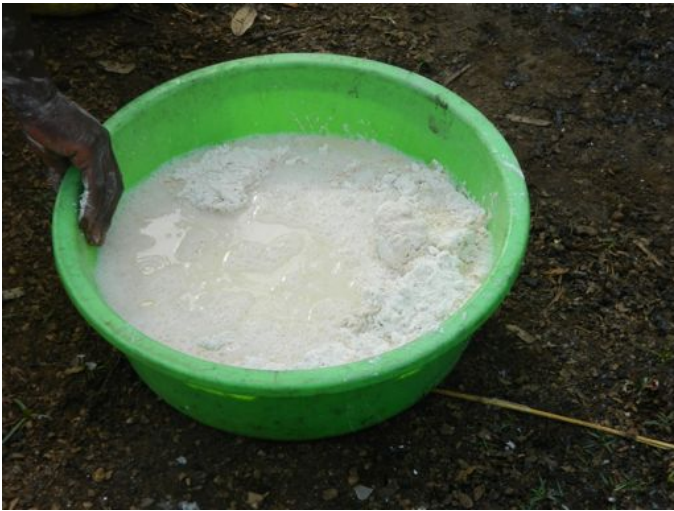
8. Ground cassava mixed with water to be used as binder
