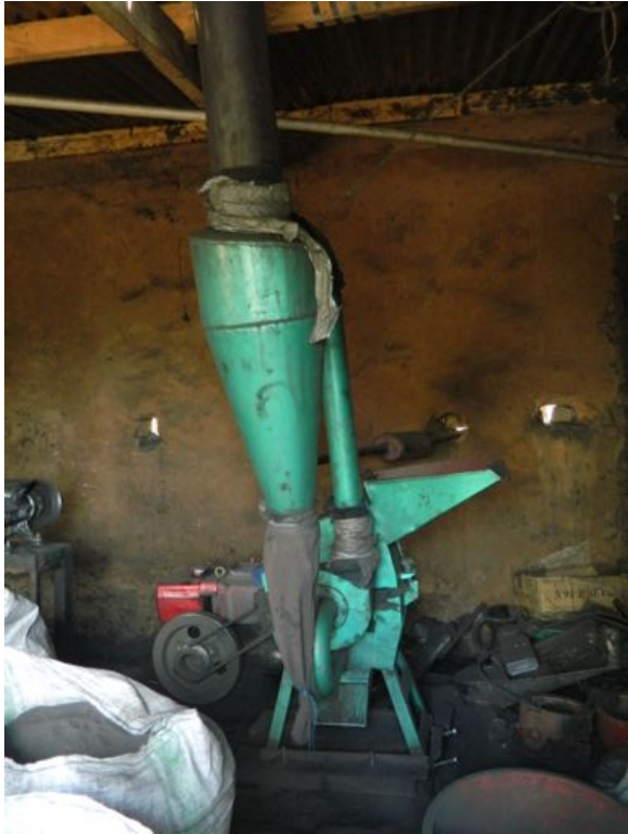
7. Posho mill machine converted to grind charcoal dust
