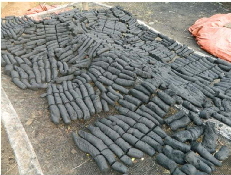
14. Briquettes put out to dry
