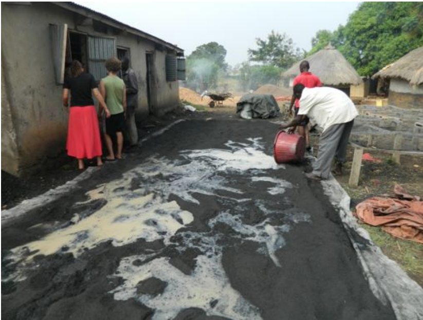
10. Binder poured on carbonized husks and charcoal dust
