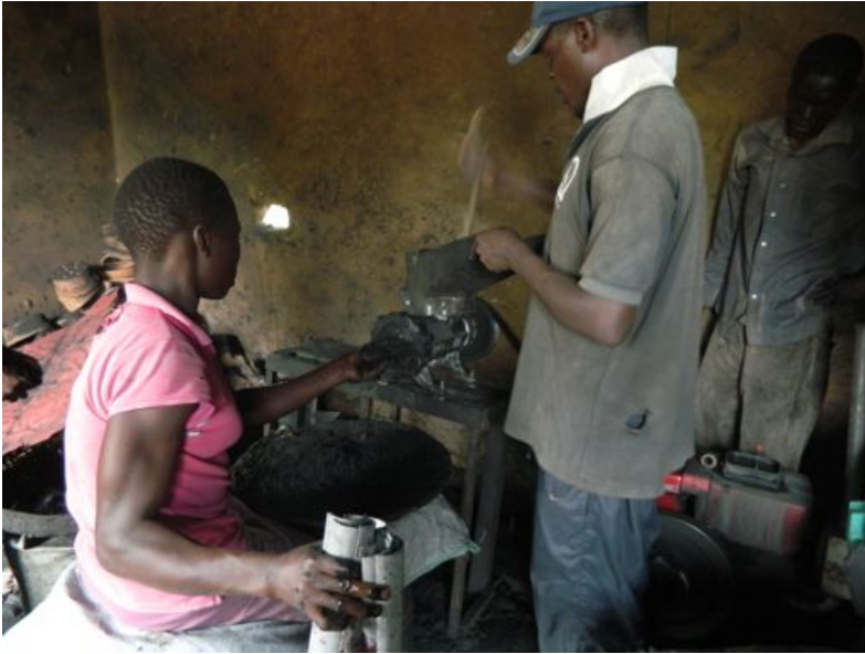
13. Mixture with binder poured into extruder converted from a meat mincer
