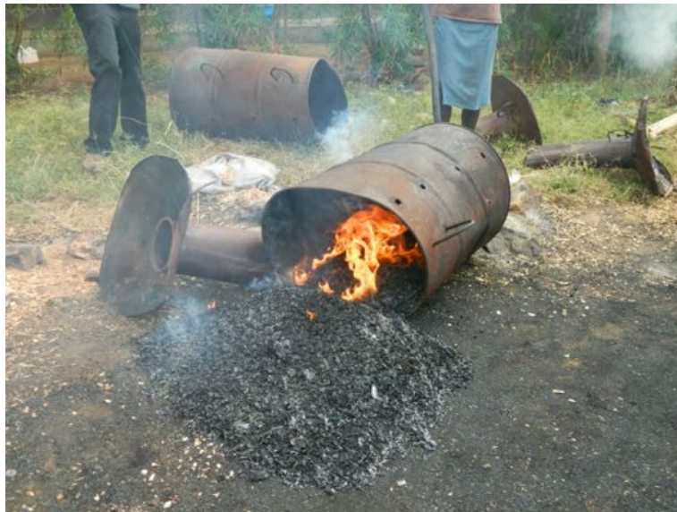
4. Fire put out after carbonization.
