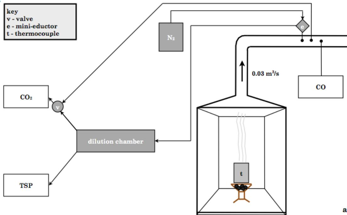
Fig. 3. Experimental set-up of the laboratory-grade combustion chamber for testing particulate and carbon monoxide emissions from the briquettes (reproduced from Banzaert, 2013).
