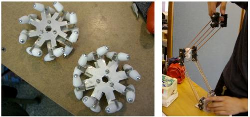
(a) Omnidirectional wheels (32 moving parts) (b) Crane (38 moving parts)
