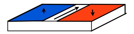
Topological band insulator: Charged one-way mode (= edge of 2d electron IQHE)
