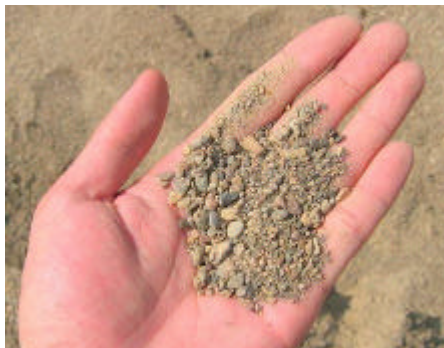
Poor coarse sand – dirty, mixed up with lots of dirt, silt, and fine sand
