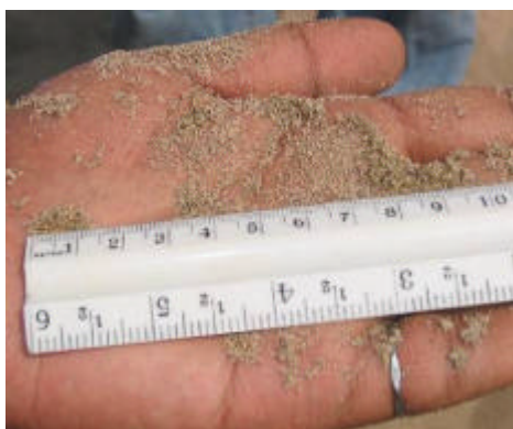
Ideal fine sand - correct size, no large particles or visual contamination
