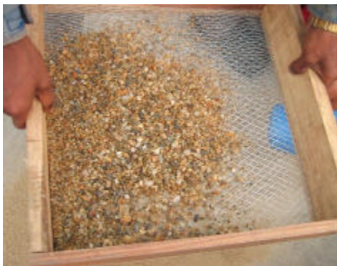
Ideal coarse sand - correct size, clean with no silt, dirt, small particles or other visual contaminations
