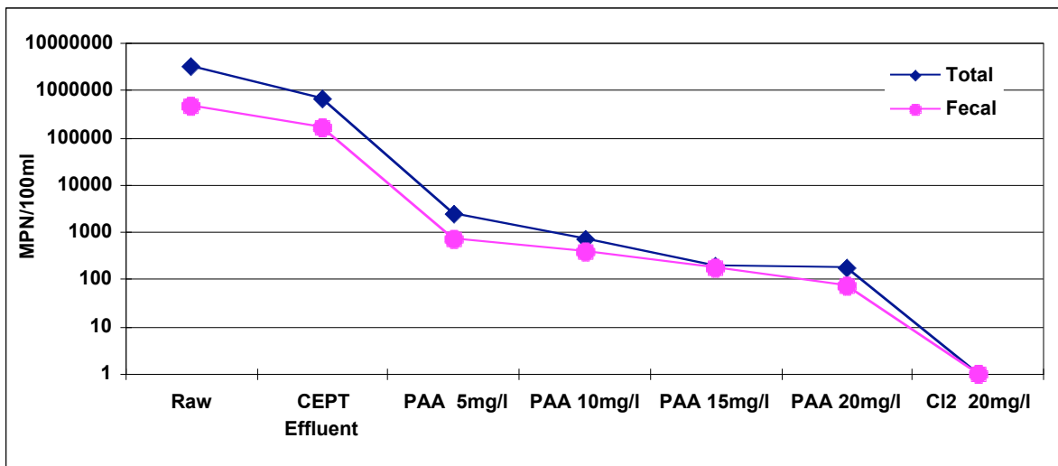
Figure I.3. Coliform reduction in CEPT effluent by PAA and chlorine
