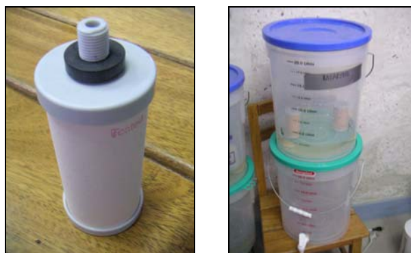
Figure 5: A Katadyn ceramic drip candle (left). The Katadyn filter system built by the MIT team in Peru (right).
