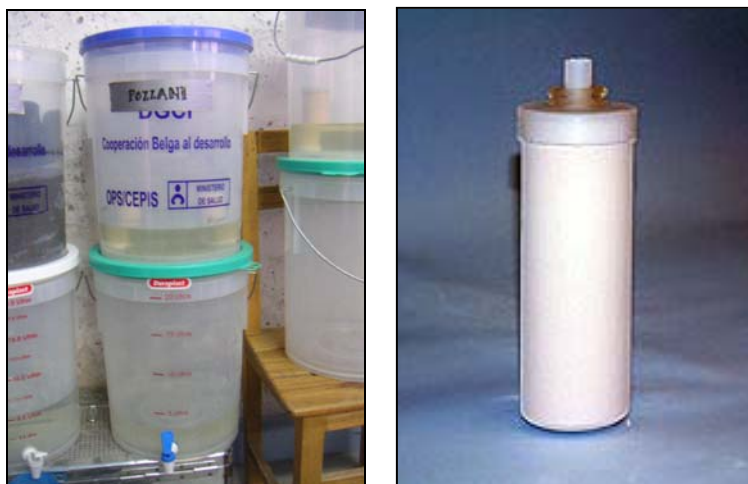
Figure 4: The Pozzani filter system built by the MIT team in Peru on the left. A ceramic Pozzani candle is pictured on the right. 5
