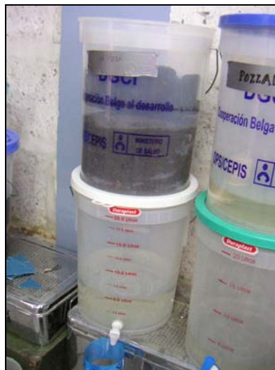
Figure 7: The Filtro de Mesa filter system built by the MIT team in Peru.
