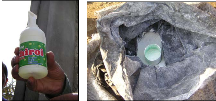
Figure 12: Pictures of chlorine added to the water for disinfection. Liquid chlorine, occasionally used for home disinfection, pictured on the left, and powder chlorine used at the CBV water treatment plant on the right.
