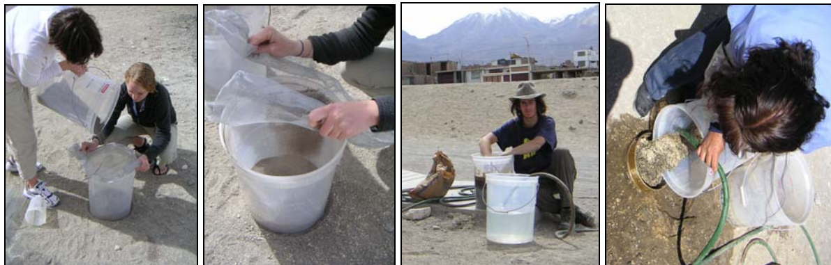
Figure 9: Sifting (left 2 pictures) and washing sand (right two pictures) for the HSSF. Photos taken adjacent to the Clinic of the Sociedad Misionera de San Pablo, Enace, Alto Cayma.
