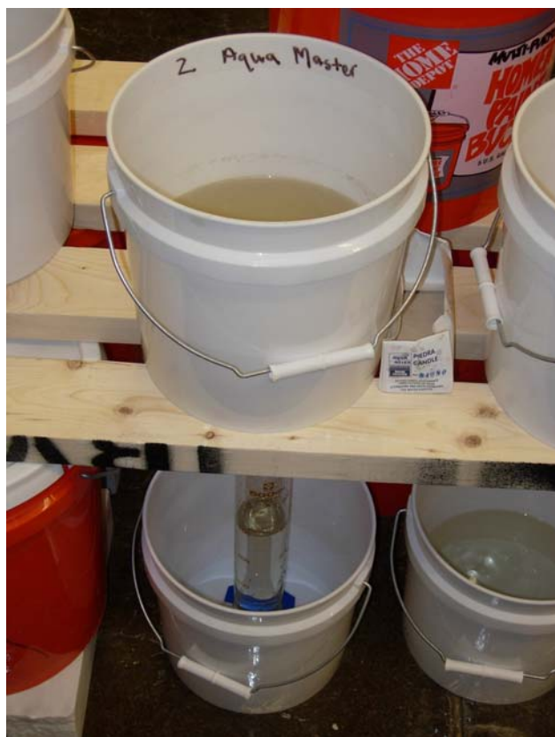
Figure 4.5: Picture Depicting Flow Rate Test via Collection of Water in Graduated Cylinder
