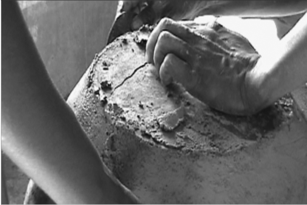
Figure 11-4: Cracked base. Cracks formed in base of vessel during firing, Amilo-Rangwe.
