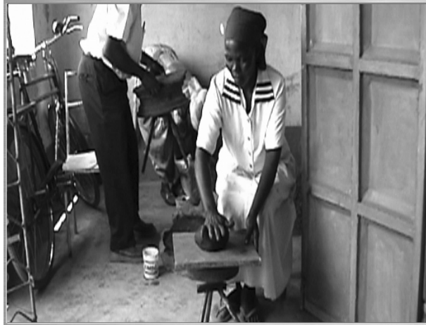
Figure 4-8: Potter, front, begins forming base. Pounds clay into flat disc.
