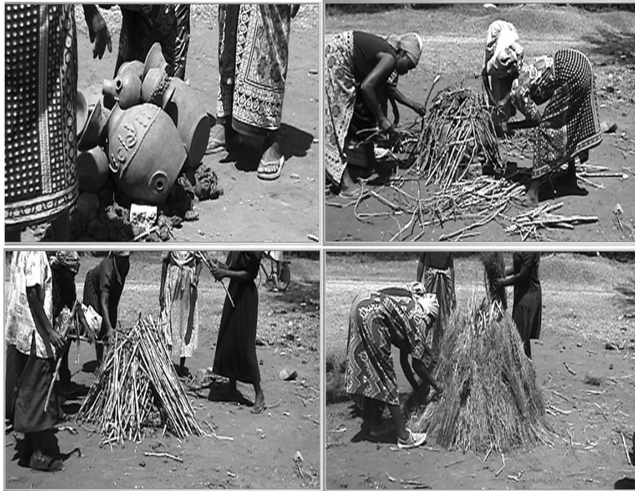
Figure 8-2: Oriang fire building process. Chronological order: top left vessels are stacked on the brick bed. Top right, slow burning fuel placed on top. Bottom left, more stacking of slow burning fuel. Bottom right, additional covering layer of fuel is added.
