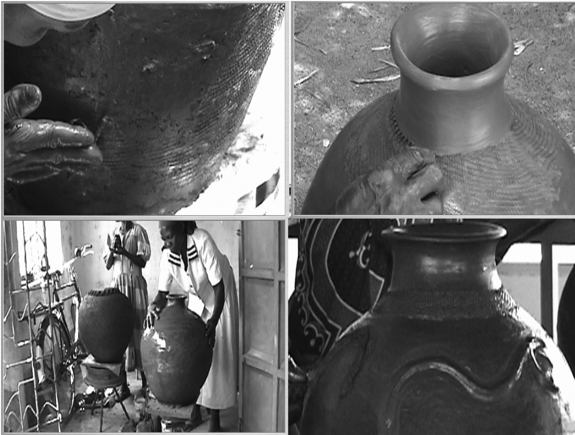
Figure 5-1: Decoration Techniques. Clockwise from top left: Impression using a kuga, Punctuation using the tip of a kuga, smoothing using the hands, and addition of clay.
