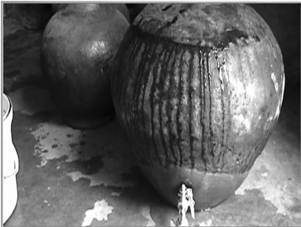
Figure 11-5: Decoration defect. A deep incision during decoration near the top of the vessel, causes excessive leaking, when the vessel is filled to the top.
