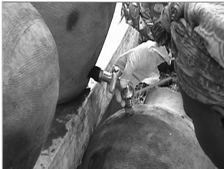
Figure 10-6: Tap stabilization. Tap wedged in vessel using another clay vessel and shards for support.
