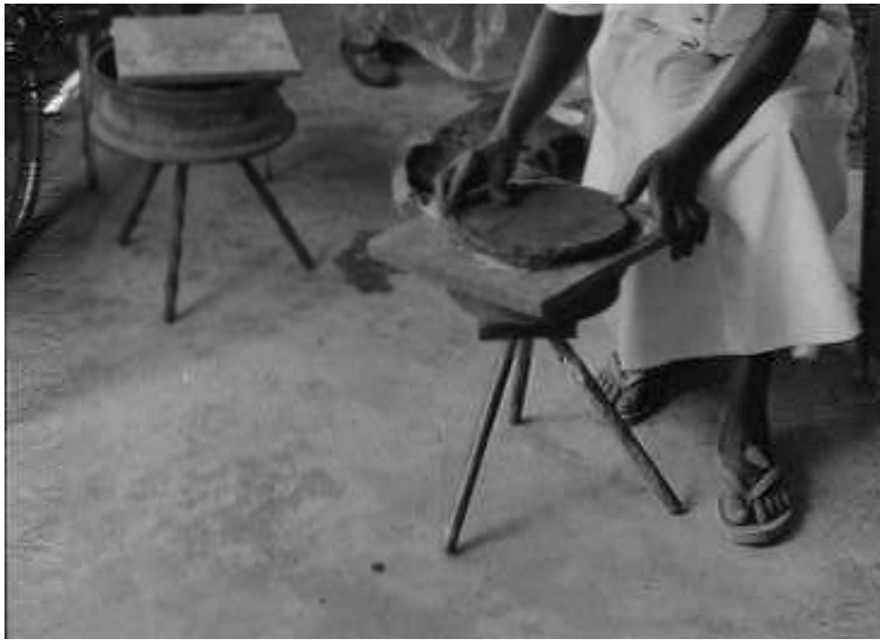
Figure 4-3: Two potter's wheels. Constructed from hubcaps mounted on a bearing welded to a metal tripod.
