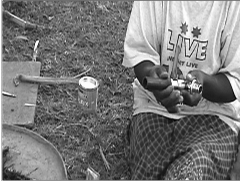
Figure 10-3: Fitted tap. Press-fitted PVC tubing to tap threads using thermal press fitting at Oriang.
