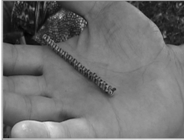
Figure 4-1: Kuga made from plastic strapping. Used by Kinda E Teko potters.
