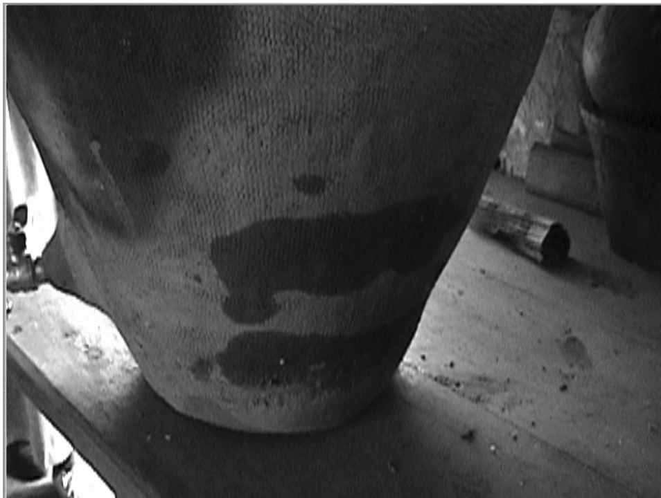
Figure 11-2: High porosity regions. Dark patches form as water permeates to surface.
