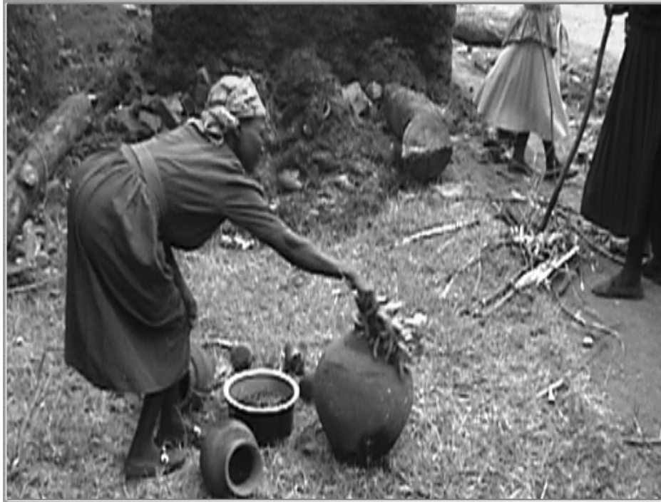
Figure 9-2: Application of orwech . Amilo-Rangwe potter uses branch to apply orwech sealant to hot vessels.
