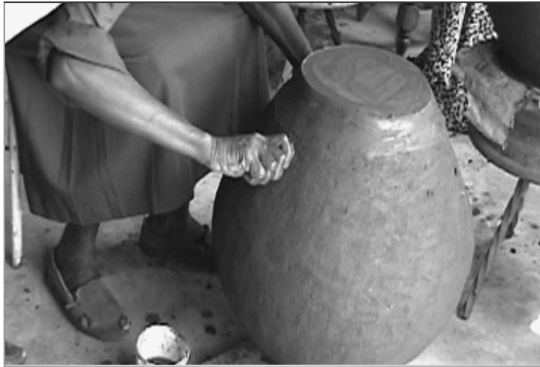
Figure 7-2: Amilo-Rangwe potter tapping a clay vessel. Potter uses 1" diameter PVC tubing to create initial opening.
