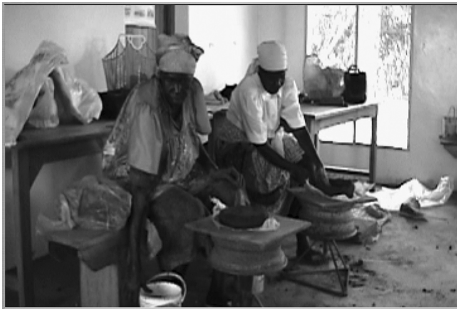
Figure 4-4: Oriang potter forms base of vessel on wheel.
