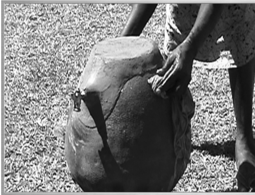
Figure 10-9: Extension of base covering. Nill layer is extended up to the tap and around the base of the vessel.
