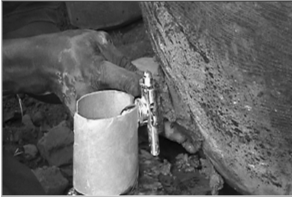
Figure 14-1: Stabilization tool. Carboard tube used to stabilize tap during attachment instead of stones and shards.
