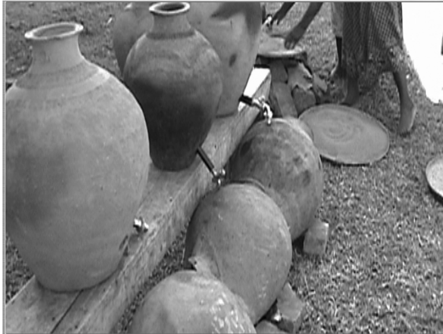
Figure 10-5: Tap attachment in parallel. 3 vessels being prepared for tap attachment in parallel.
