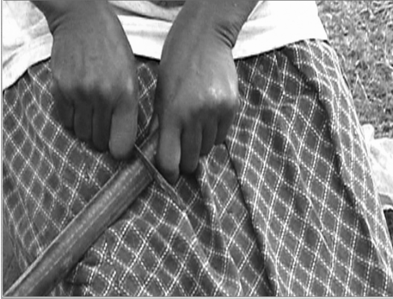
Figure 10-1: PVC tube cut to length. Oriang putter cutting PVC tubing to length with a hacksaw blade.
