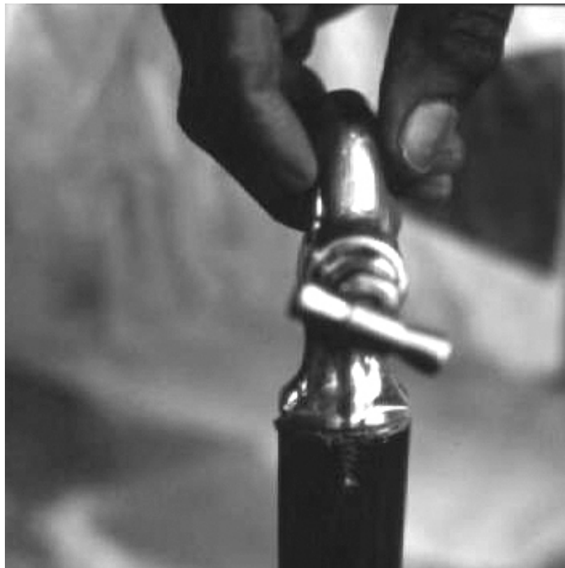
Figure 10-4: Closeup of split PVC pipe. Used by Kinda E Teko potters to fit tap to PVC tubing.
