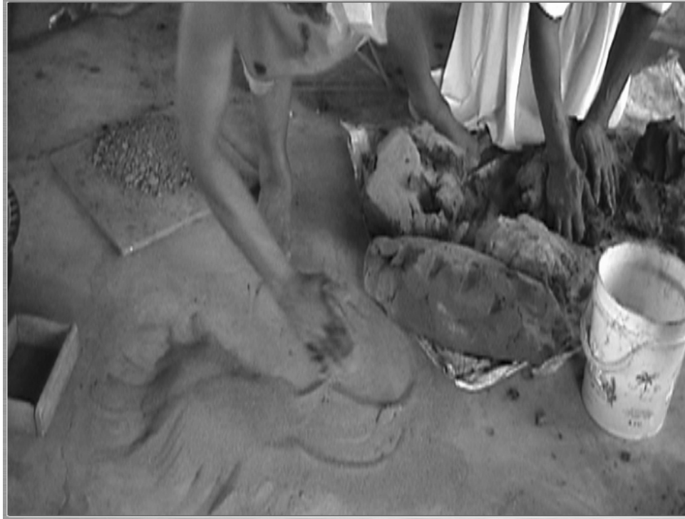
Figure 3-3: Oriang potters tempering clay with sand.
