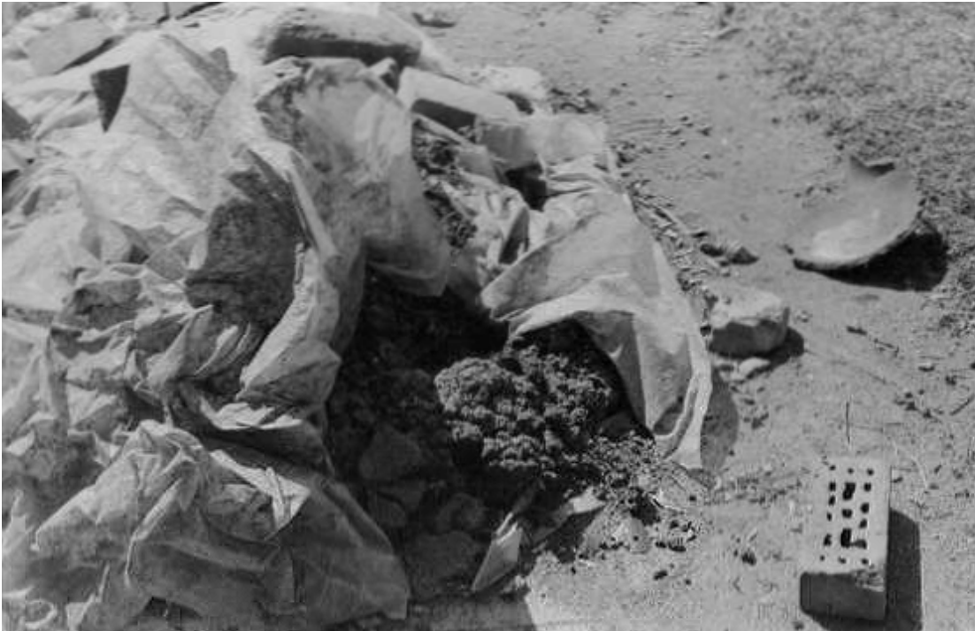
Figure 3-1: Aging clay at Oriang. The clay is covered with plastic tarp and bricks to prevent drying out.
