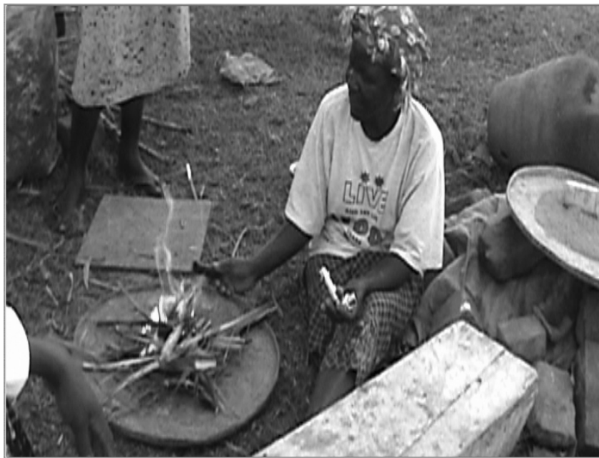
Figure 10-2: Thermal press-fitting. Oriang potter heating PVC to press fit to tap threads.
