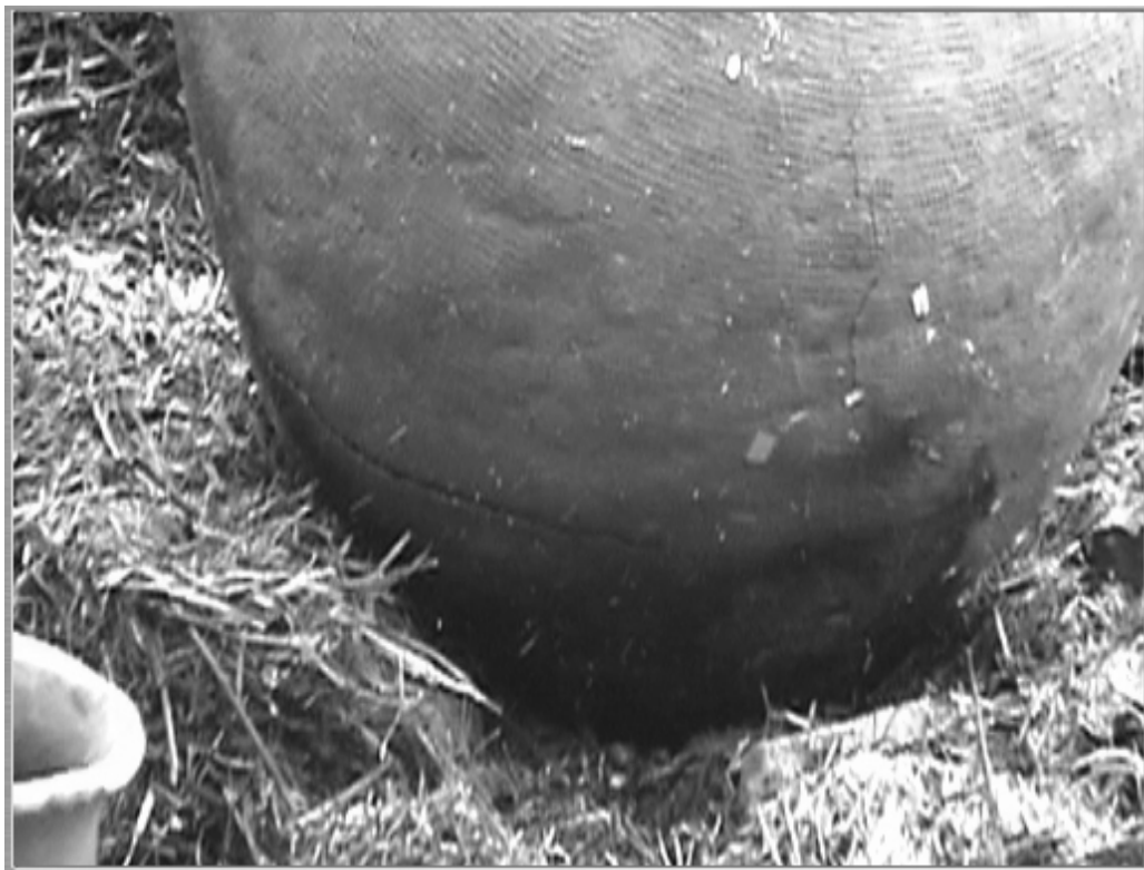
Figure 11-3: Firing defects. Cracks formed in vessel after firing at Amilo-Rangwe.
