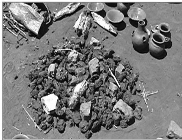
Figure 8-1: Brick mound. Used for open firing at Oriang.
