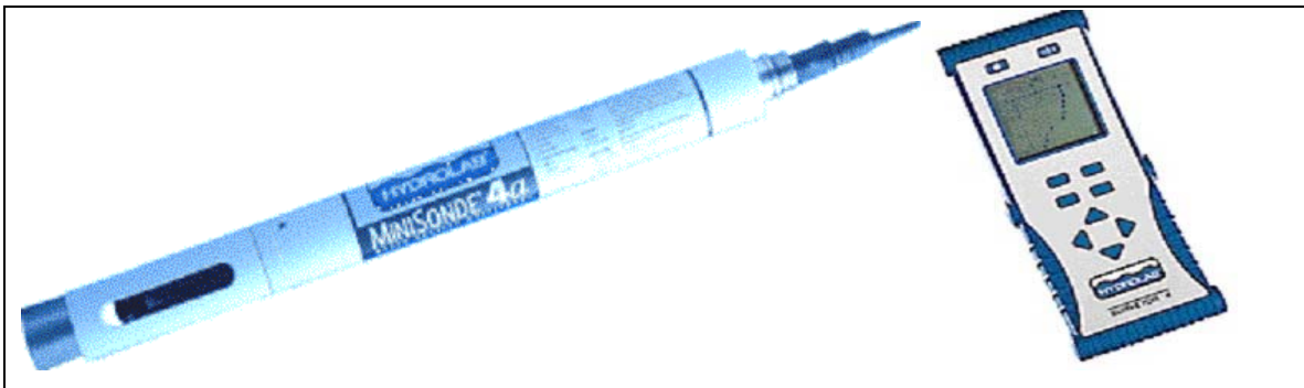
Figure 4.4: Hydrolab: The MiniSonde® 4a Electrode (Left) and the Hydrolab hand-held Surveyor® 4a Meter (Right).
