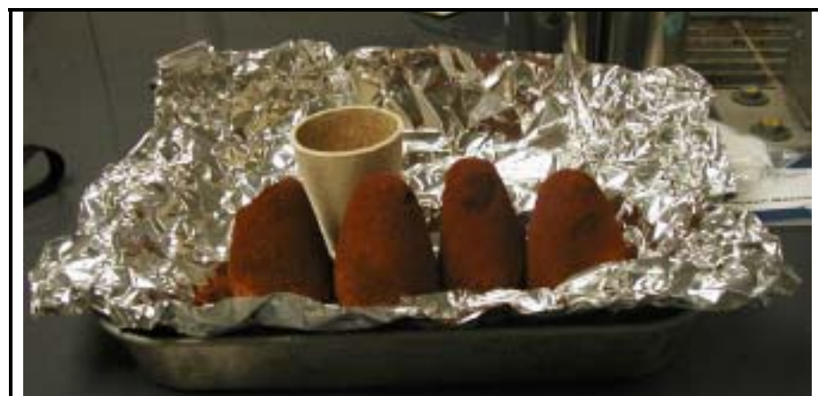
Figure 4.5 Dried sand after heating at 550°C.
