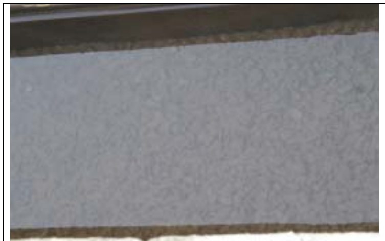
Figure D.3 Iron oxide coated gravel in Laxmipur ARP (top view as seen through water).
