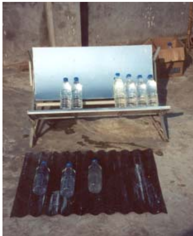
FIGURE 6.10: SODIS IN LUMBINI USING THE SOLAR MIRROR AND BLACK SHEET METAL
