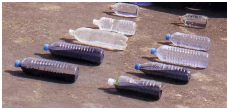
Figure 10.1: Experiment on the Effectiveness of SODIS using Different Bottles, Some with Black Backs. Source: Khayyat, 2000.
