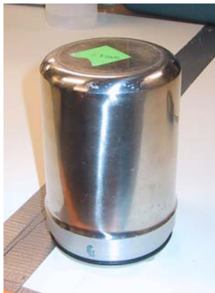
Figure 7.5: Millipore Portable Membrane Filtration Filter Holder with Lid Closed for Sterilization
