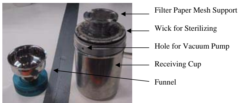
Figure 7.7: MF Filter Holder Showing the Filter Mesh Support
