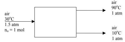
There is no net heat or work interaction with the surrounding. Assume air is an ideal gas with Cp = 3.5R (constant). Is the process drawn above feasible?
