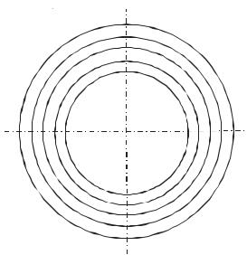
Consider a cylindrical multi-layered composite beam made up of hollow cylindrical beams of different *brittle* materials with Young's moduli;  $E_1 = 4E$ ,  $E_2 = 3E$ ,  $E_3 = 2E$ ,  $E_4 = E$ . E = 400 GPa. The internal radius of cylinder 1 is a = 25 mm, while all hollow cylinders are of thickness t = 2.5 mm. Observe a > t. The fracture strengths are;  $\sigma_f^1 = 2\sigma_f$ ,  $\sigma_f^2 = \sigma_f$ ,  $\sigma_f^3 = 0.5\sigma_f$ ,  $\sigma_f^4 = 0.25\sigma_f$   $\sigma_f = 25$  MPa
