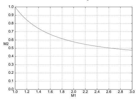
The  $M_1 \to 1^+$ ,  $M_2 \to 1^-$  limit corresponds to infinitesimal shock, or a sound wave. The  $M_2(M_1)$  function is not shown for  $M_1 < 1$ , since this would correspond to an "expansion shock" which is physically impossible based on irreversibility considerations.
