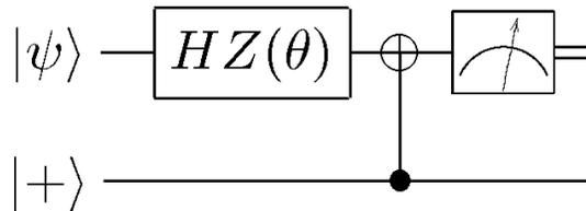
Define  $|\tilde{\psi}\rangle = HZ(\theta)|\psi\rangle$ . Compare this circuit with the second one in problem 2 we can see that the output state is  $|\tilde{\psi}\rangle$  up to classically controlled  $X$  operation. Therefore the output is  $X^m |\tilde{\psi}\rangle = X^m HZ(\theta)|\psi\rangle$ .
