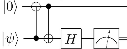
The two CNOT gates swaps the two qubits. Obviously,  $|\psi\rangle$  is output on the first line.
