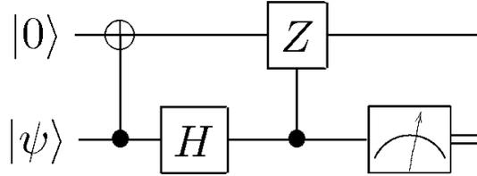
Control-Z operation is symmetric between control bit and target bit, hence the circuit is equivalent to
