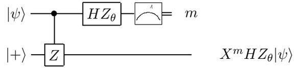
is a qubit in the state  $X^m HZ_\theta |\psi\rangle$ , where  $m$  is the measurement result. This is a key idea used in the cluster model of QC. How is this construction related to teleportation?
