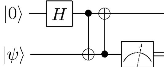
The two CNOT gates swaps the two qubits. Obviously,  $|\psi\rangle$  is output on the first line.
