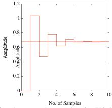
K=2.0 On the negative real axis: Yield oscillations Settling time = 7 T Prediction =  $4/\ln(0.55) = 7$ Predicted damping = 0.2 therefore overshoot expected.
