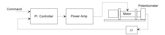
Use the function generator and the oscilloscope to record the step response of this system. Explain your observations in terms of a root-locus.
