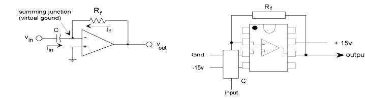
Use a 4.7  $\mu$ F capacitor and a 10K resistor. Compute the transfer function of the differentiator.
