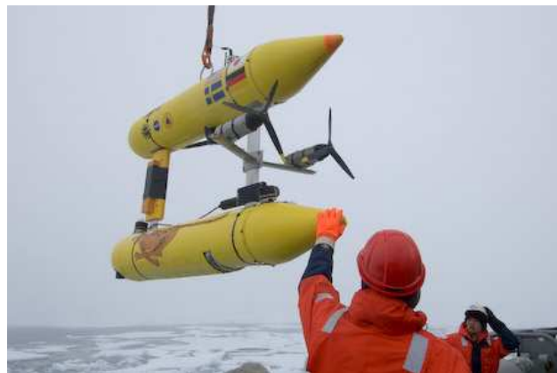
Figure 2: The Jaguar AUV being brought back on deck after a mission.
