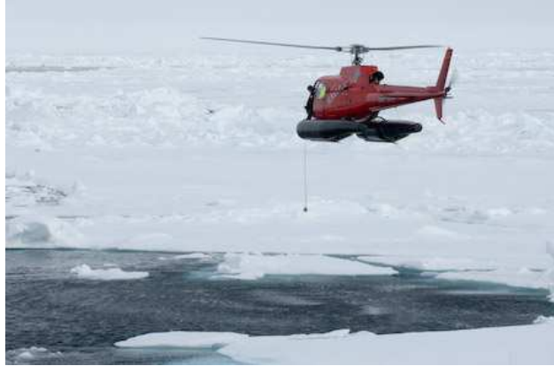
Figure 4: Hydrophone being lowered into an open lead during a helicopter survey of a long baseline transponder’s location on the seafloor approximately 4000 m below. Acoustic ranges were opportunistically collected at 5–6 open leads per transponder. A GPS receiver on board the helicopter enabled geo-referencing of the survey positions and ultimately of the sub-sea transponder itself.
