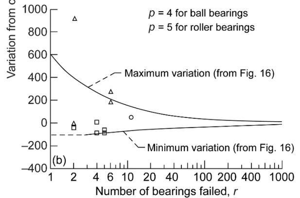
Figure 20.—Effect of VAR AISI M-50 steel and load-life exponent on bearing life (Ref. 90). (a) Load-life exponent  $p$  is 3 for ball bearings and 10/3 for cylindrical roller bearings (from Fig. 18). (b) Load-life exponent  $p$  is 4 for ball bearings and 5 for cylindrical roller bearings.
