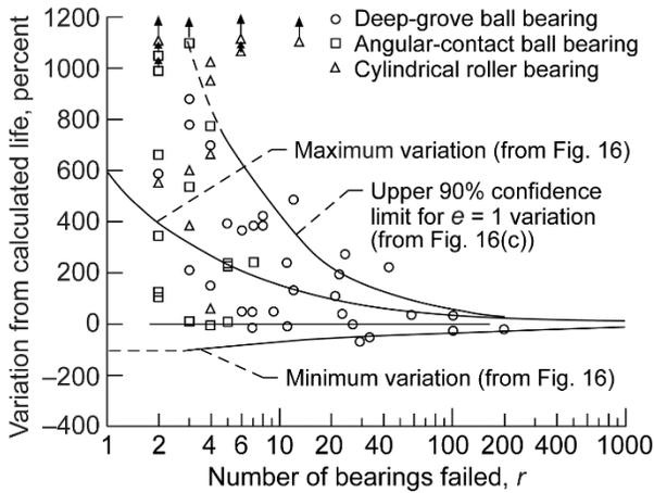
Figure 18.—Variation between actual and calculated  $L_{10}$  bearing lives for 51 sets of deep-groove and angular-contact ball bearings and cylindrical roller bearings from References 91 and 92 compared with Monte Carlo variations and 90% confidence limit (Ref. 90).
