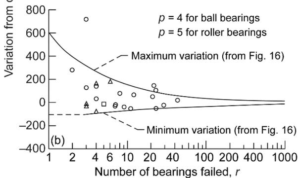
Figure 19.—Effect of CVD AISI 52100 steel and load-life exponent on bearing life (Ref. 90). (a) Load-life exponent  $p$  is 3 for ball bearings and 10/3 for cylindrical roller bearings (from Fig. 18). (b) Load-life exponent  $p$  is 4 for ball bearings and 5 for cylindrical roller bearings.
