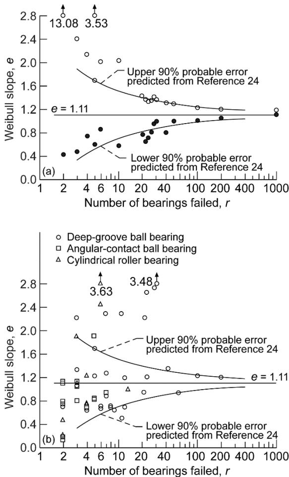
Figure 23.—Variation of Weibull slope  $e$  compared with predicted 90% probable error. (a) Extremes of Weibull slope from Monte Carlo testing for each group of 10 bearing trials of  $r$  bearings (data from Ref. 90). (b) Weibull slopes from 51 sets of ball and roller bearings (data from Refs. 91 and 92).
