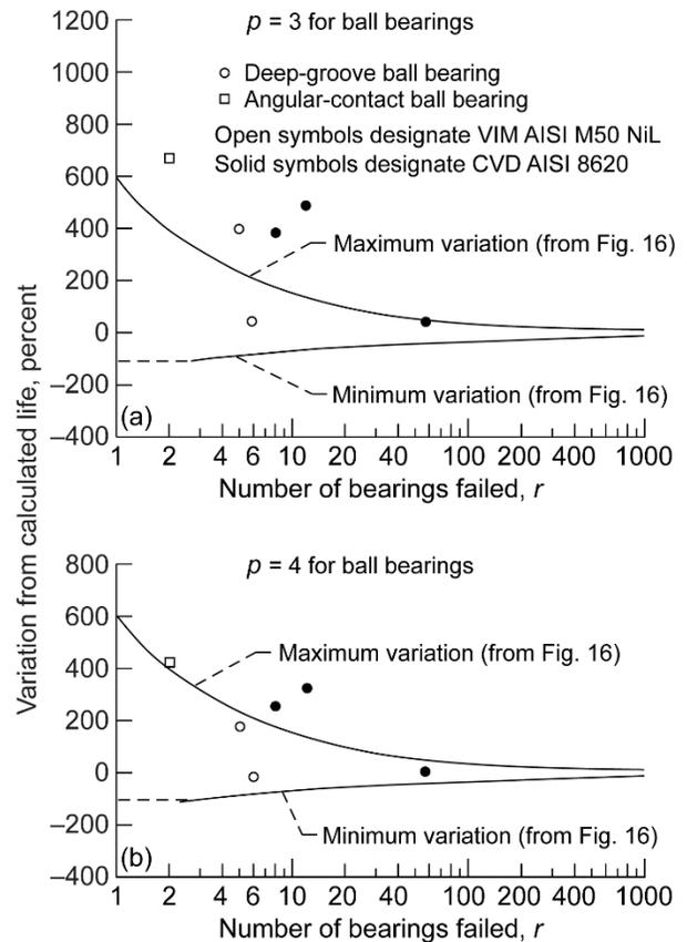
Figure 22.—Effect of VIM–VAR M50 NiL and CVD AISI 8620 steels and load-life exponent on bearing life (Ref. 90). (a) Load-life exponent  $p$  is 3 for ball bearings (from Fig. 18). (b) Load-life exponent  $p$  is 4 for ball bearings.
