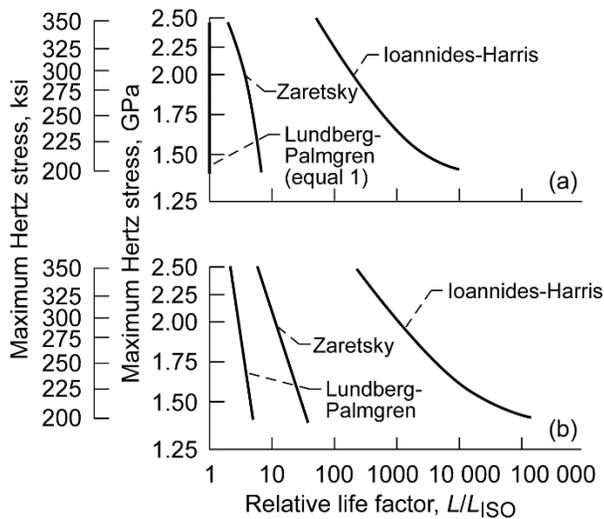
Figure 15.—Comparison of life models for rolling-element bearings with ANSI/ABMA and ISO standard without a fatigue limit. Fatigue-limiting shear stress for  $\tau_{45}$  assumed for Ioannides-Harris model, 276 MPa (40 ksi) (Ref. 85). (a) Ball bearings. (b) Cylindrical roller bearings.
