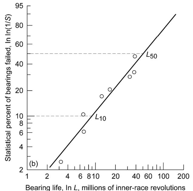
Figure 1.—Weibull plot where (Weibull) slope of tangent of line is  $e$ ; probability of survival  $S_{\beta}$  is 36.8 percent at which  $L = L_{\beta}$ , or  $L/L_{\beta} = 1$ . (a) Schematic where  $S$  is probability of survival. (b) Rolling-element bearing fatigue data where  $\ln \ln(1/S)$  is presented in ordinate as statistical percent of bearings failed.
