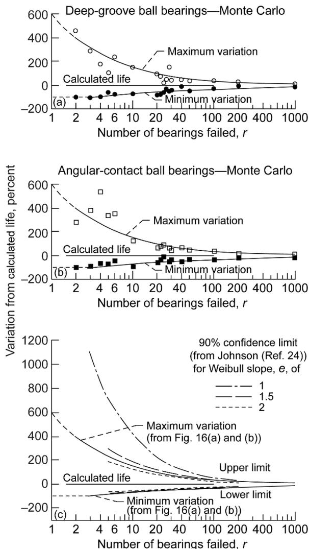
Figure 16.—Maximum and minimum variation of  $L_{10}$  lives as percent of calculated  $L_{10}$  for groups of  $r$  bearings and 90% confidence limits based on Weibull slope and number of bearings failed  $r$  (Ref. 90). (a) 50-mm-bore deep-groove ball bearing. (b) 50-mm-bore angular-contact ball bearing. (c) 90% confidence limits.
